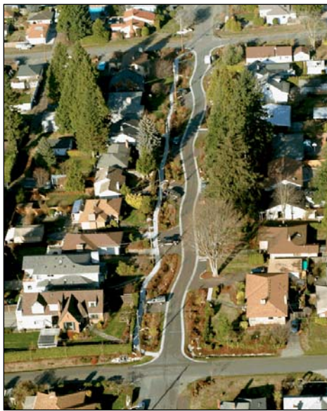
Figure 4. An aerial view of “Street Alternative Edge” design showing narrow, curvilinear streets with sidewalks and street-edge gardens.
