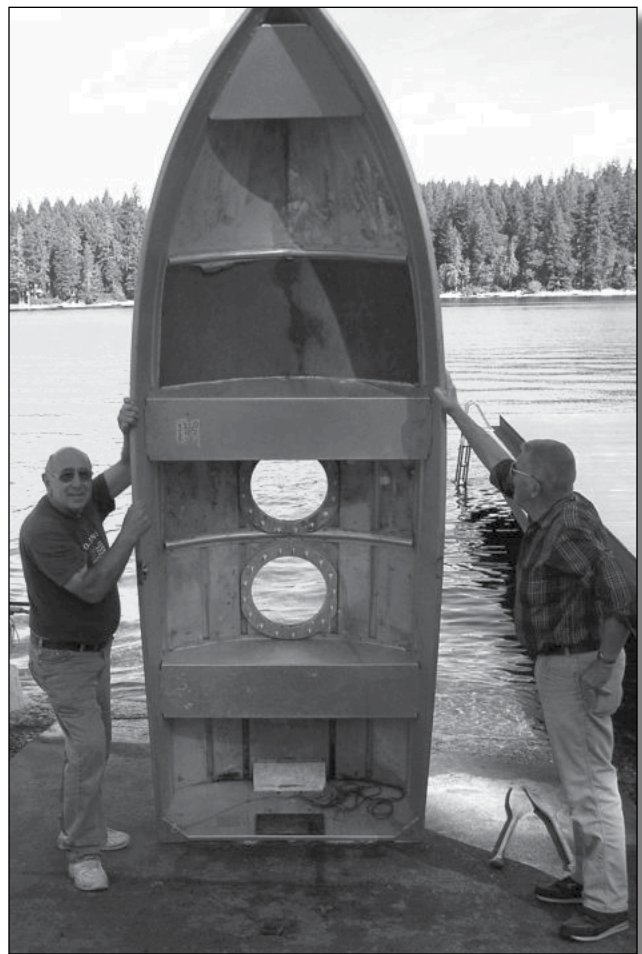
A boat has been modified to have a “glass bottom” for use surveying for aquatic noxious weeds on Mason Lake.
