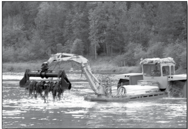
A mechanical harvester removes Eurasian watermilfoil from the Pend Oreille River during a September, 2004 tour.
