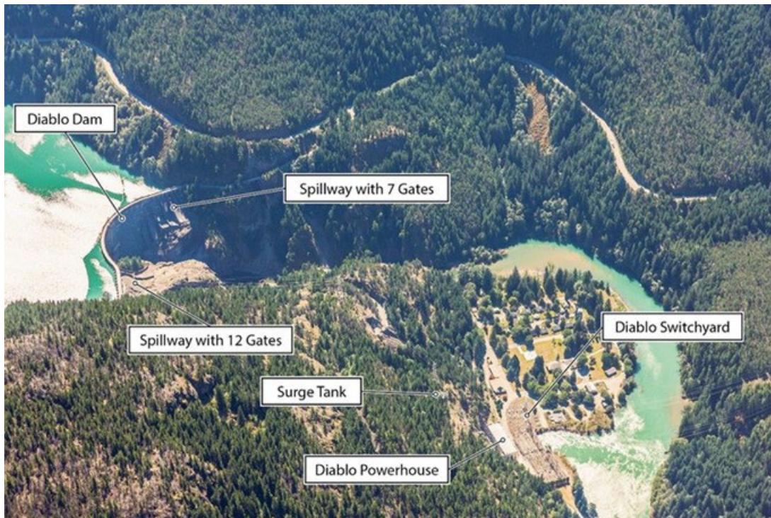
Figure 5.0-2. Aerial view of Diablo Development and associated facilities (not visible in photo: intake on right bank and valve house on face of the dam).
