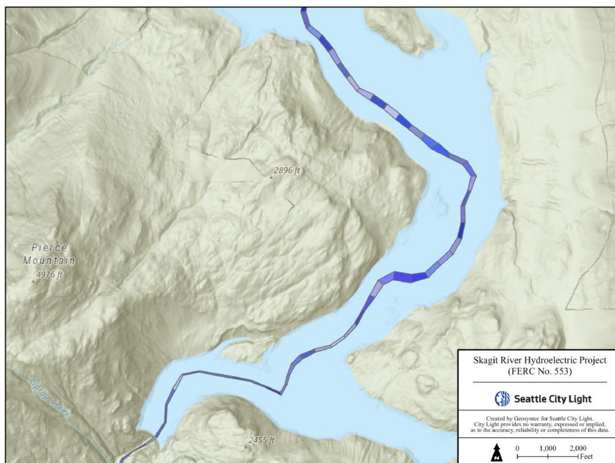
Figure 4.5-2. Example model segmentation of the Without-Dams Simulation Skagit River in present-day Ross Lake. Shading differentiates segments from one another visually and does not indicate differences between segments.
