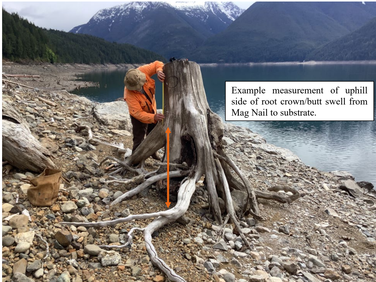
Figure 4.2.1-7. Measurement of erosion around exposed stumps.
