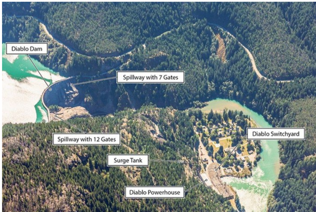
Figure 3.1-3. Aerial view of Diablo Development and associated facilities (not visible in photo: intake on right bank and valve house on face of the dam).
