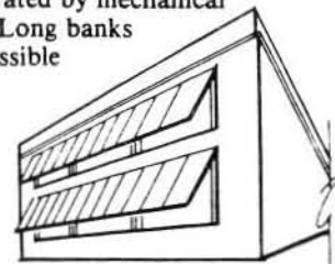
Fig. 4 Typical rolled steel windows available from 1890 to the present. The various operating and ventilating capacities in combination with the aesthetics of the window style were important considerations in the selection of one window type over another. Drawings: Sharon C. Park, AIA.
