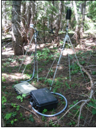
Figure 14. Acoustic monitoring equipment at the Thornton Lakes Trail site (NOCA021).
