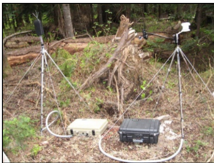
Figure 12. Acoustic monitoring equipment at the Beaver Pass site (NOCA019).
