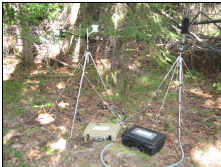
Figure 13. Acoustic monitoring equipment at the Stehekin Airstrip site (NOCA020).
