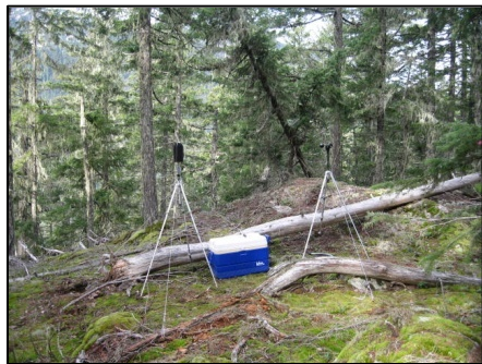
Figure 6. Acoustic monitoring equipment at the Ross Dam Trailhead site (NOCA012).
