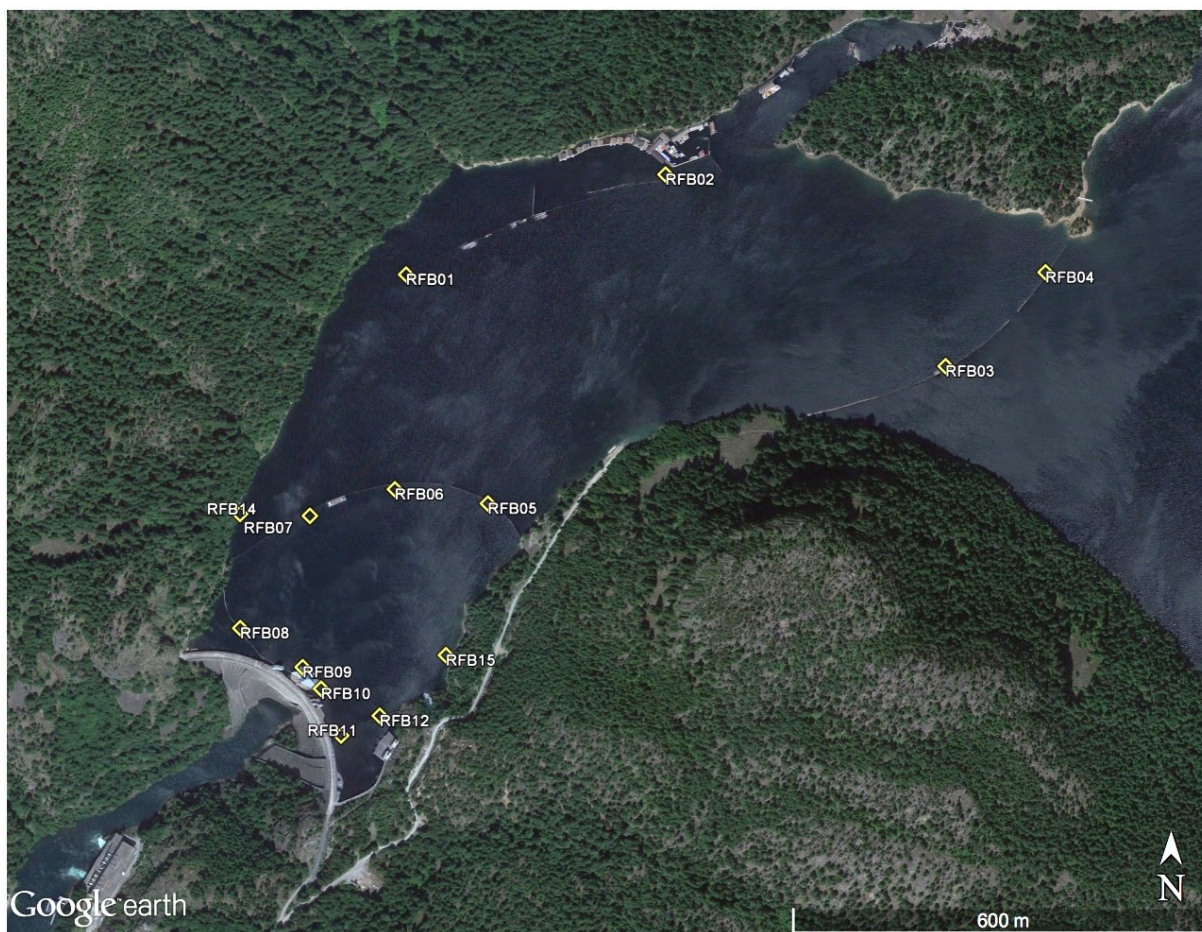
Figure 1. Acoustic receiver array in Ross Lake forebay for 2017.
