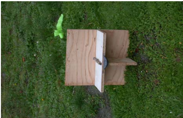
Figure D.VI.1. The drift buoy. The base is 13 inches by 13 inches, and made of plywood. The pole is a bamboo garden stake. The base has a four-ounce fishing weight attached for displacement.
