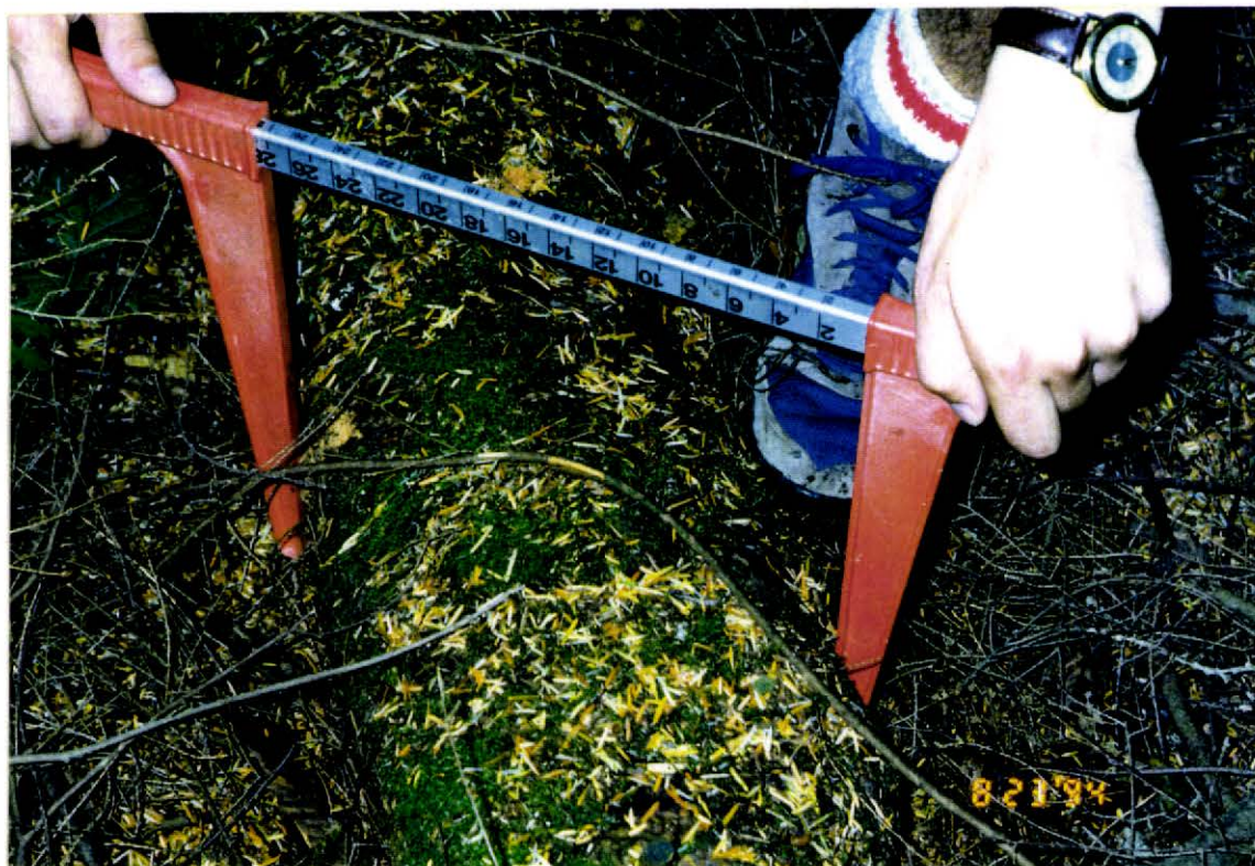
Figure 7: Using 50.0cm calipers to measure fuel with a diameter of greater than 7.0cm.
