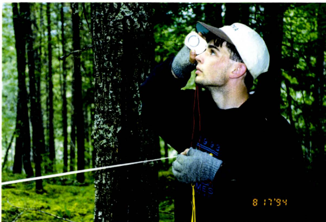
Figure 4: Determining the height of a tree using a suunto clinometer and a 50.0m chain.
