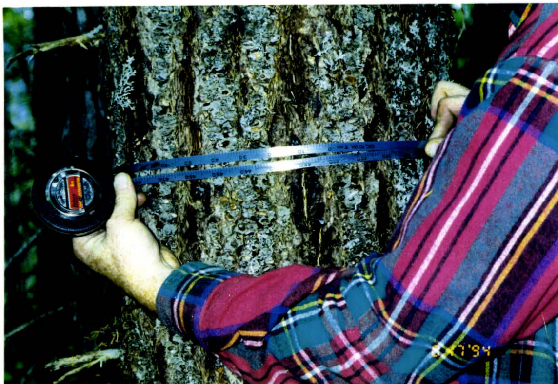
Figure 3: Using a diameter tape to measure a tree's diameter.
