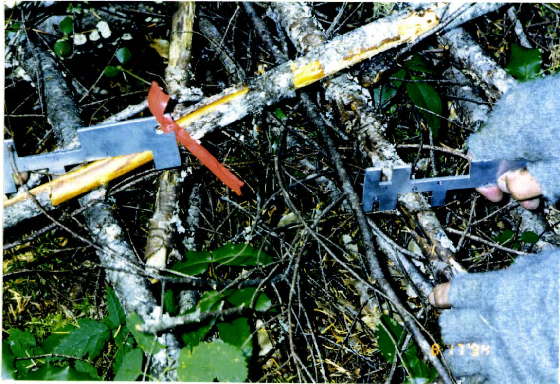
Figure 6: Using go-no-go gauges to measure the diameter class that fuel fits into.
