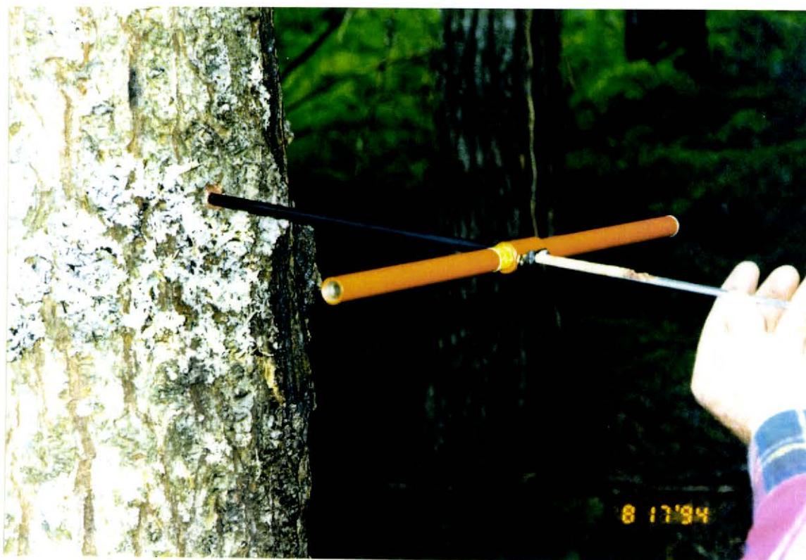
Figure 5: Using an increment bore to determine the age of a tree.
