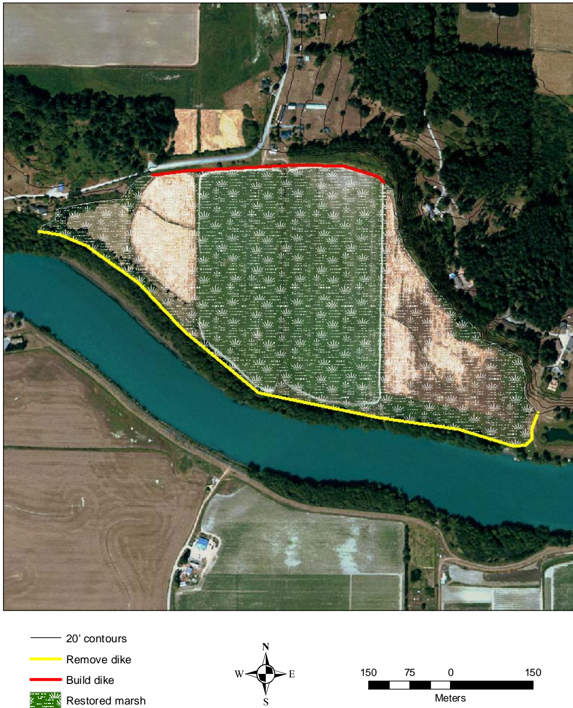
Figure 11.9. Thein Farm . Conceptual restoration design for Thein farm project. Dike reinforcement is shown in red. Dike removal is shown in yellow.
