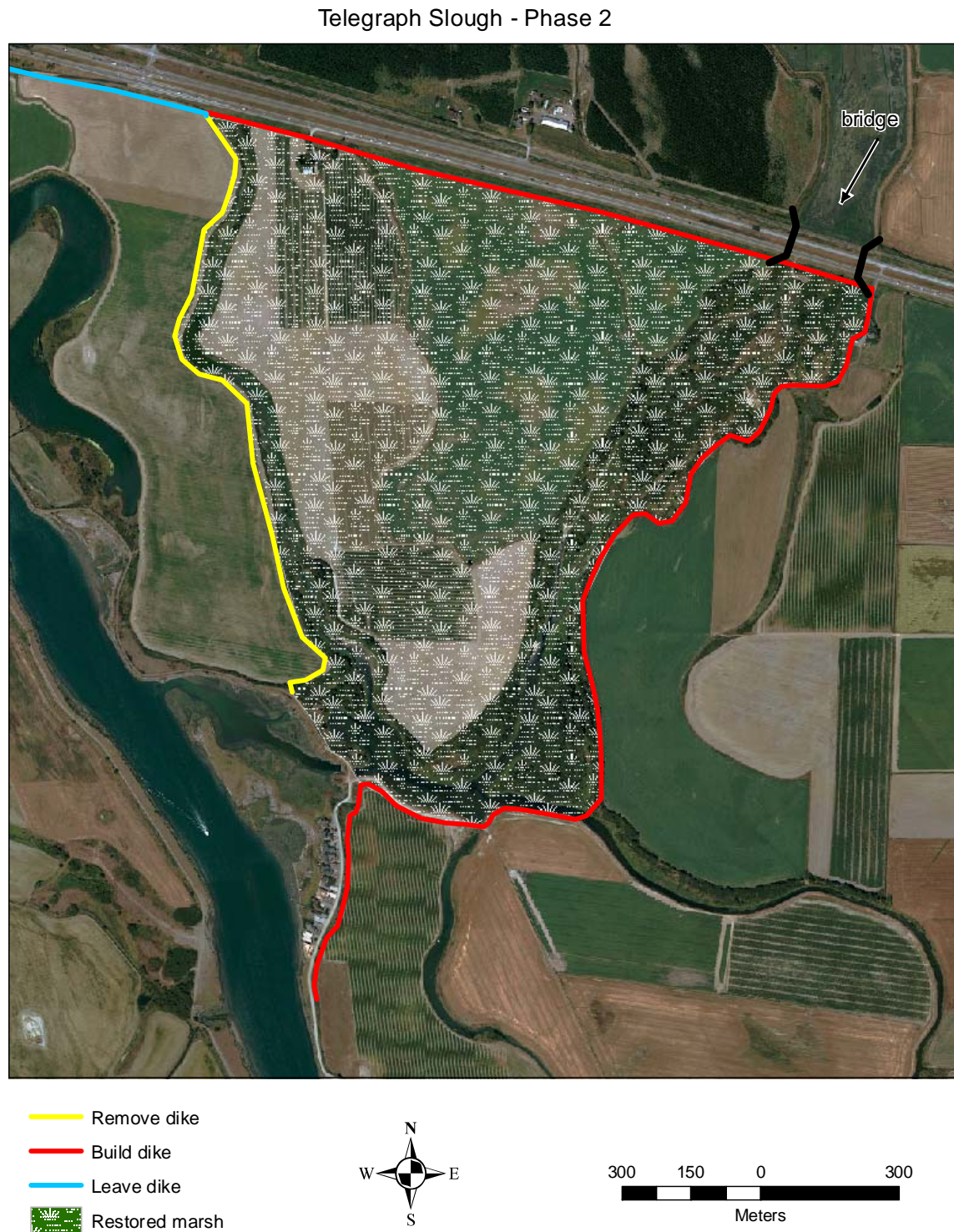
Figure 11.11. Telegraph Slough - Phase 2 . Conceptual restoration design showing levee setback and additional marsh area that would complement the area created in phase 1.
