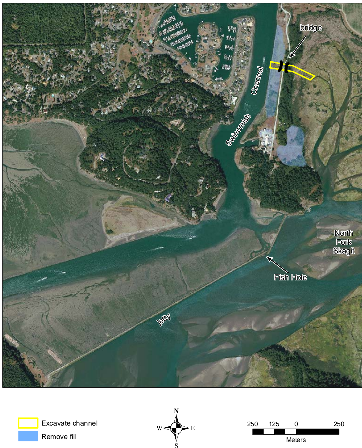
Figure 11.6 McGlinn Island . Causeway conceptual design showing potential breach location. This action would likely be accompanied by work at the existing jetty fish way.
