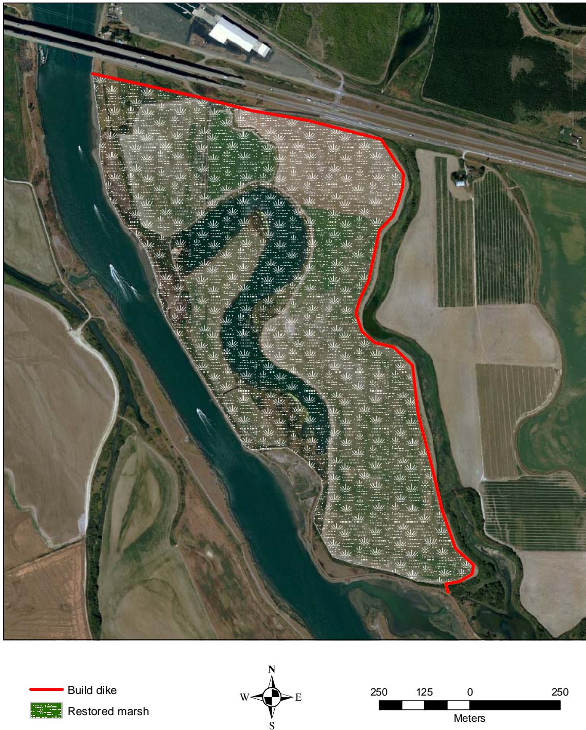
Figure 11.5 Telegraph Slough – Phase 1 . Levee set back alignment shown in red with potential emergent marsh area highlighted.
