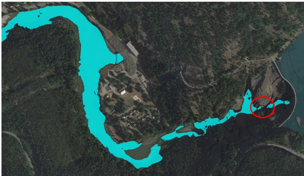
Figure 2. Initial WSE 878.5 NAVD 88 showing pockets of potential loss of connectivity within the reach above Diablo Powerhouse. Red circle identifies area where loss of connectivity in model output is likely an artifact of insufficient coverage in model DEM. Areas of loss hydraulic connectivity at downstream locations are based upon sufficient DEM coverage.
