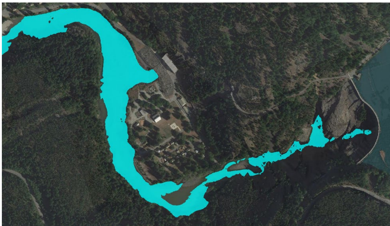
Figure 3. Initial WSE set to elevation 879 feet NAVD 88 to show connectivity within river reach above Diablo Powerhouse.
