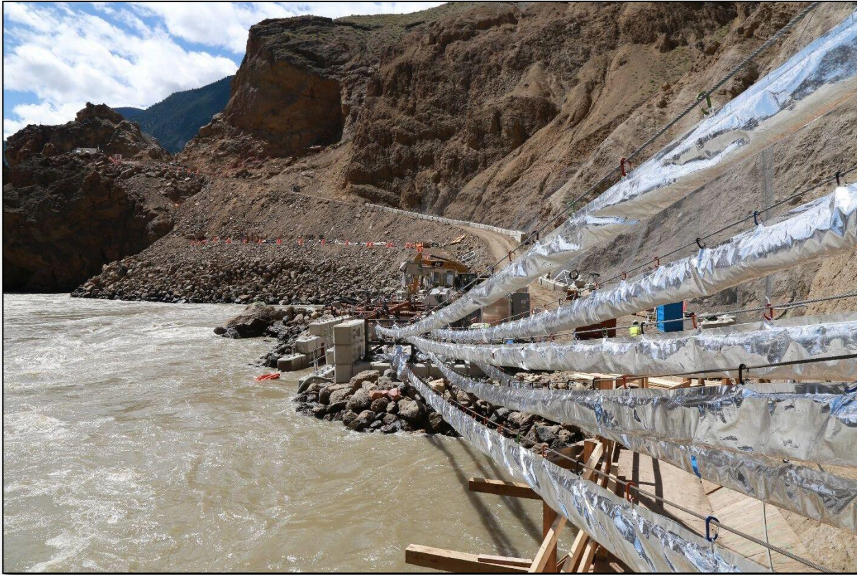
Six-lane pneumatic fish transport tube system (also known as “Whooshh”) at the Big Bar emergency fish transport site, Fraser River, British Columbia.
