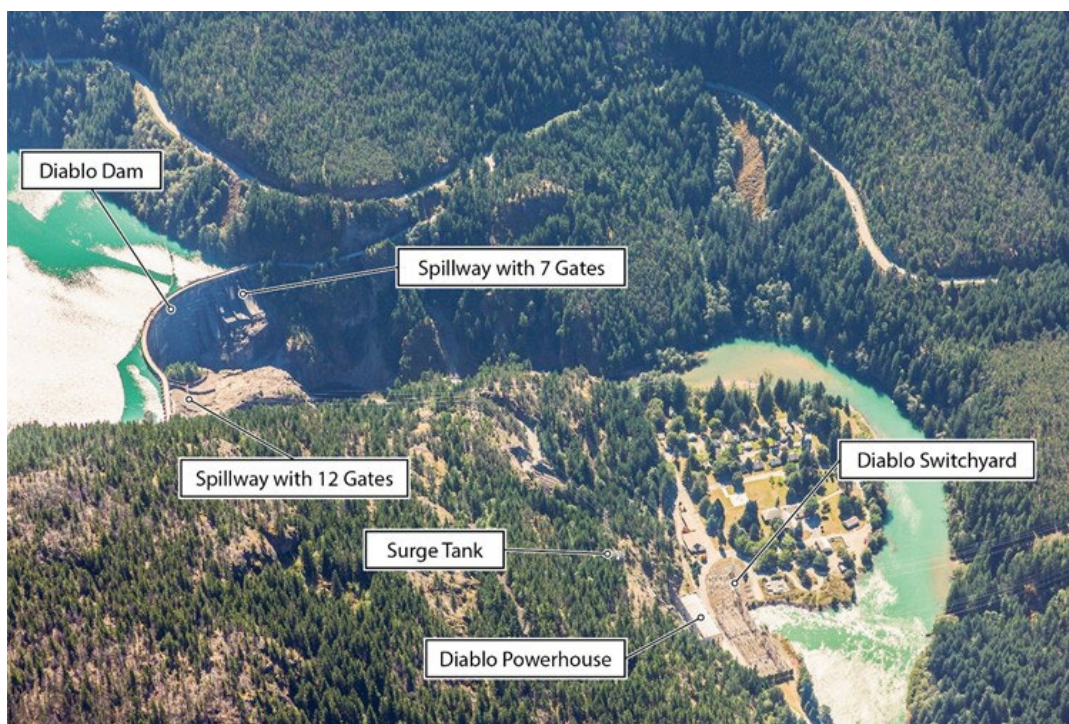
Figure 2.2-14. Aerial view of Diablo Development and associated facilities (not visible in photo: intake on right bank and valve house on face of the dam).
