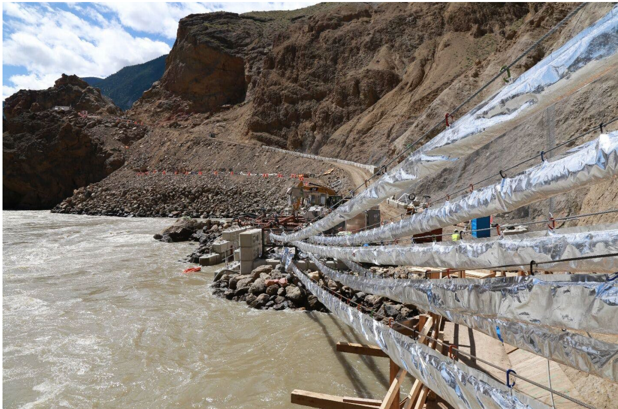
Figure 7.2-11. Six-lane pneumatic fish transport tube system (also known as “Whooshh”) at the Big Bar emergency fish transport site, Fraser River, British Columbia.
