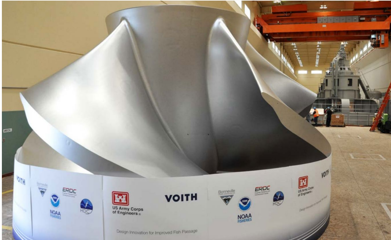
Figure 7.2-27. Example of a fish-friendly turbine used on the Ice Harbor Dam in Eastern Washington.
