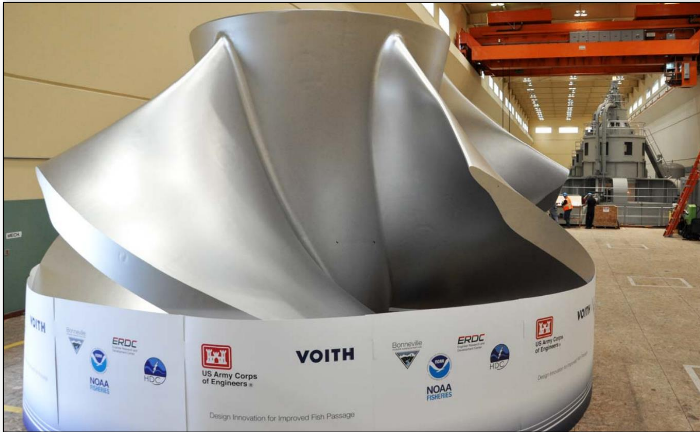
Fish-friendly turbine used on the Ice Harbor Dam in Eastern Washington.
