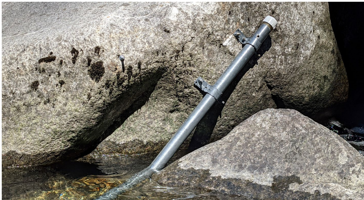
Figure 13. Mounted stilling well at Existing Feature 2.
