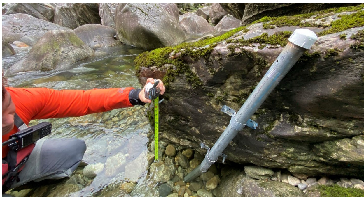
Figure 14. Distance to water reading from separate reference bolt at logger DDL3.
