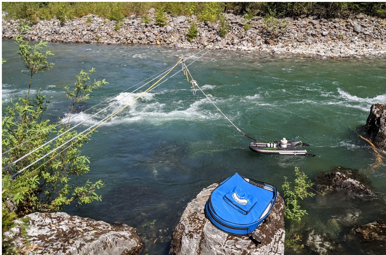
Figure 2. Cableway deployment of ADCP at Transect AA on July 26, 2021.
