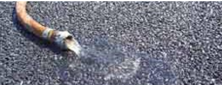
Permeable concrete lets stormwater pass through
