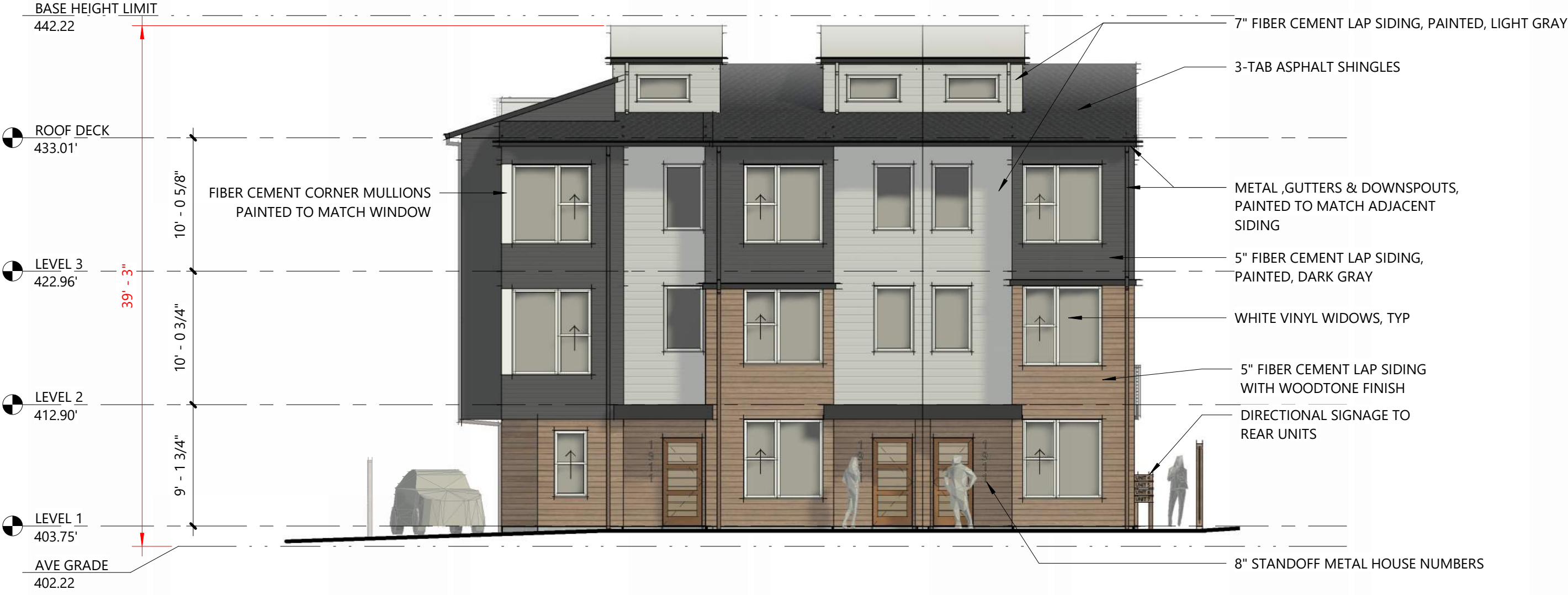
NORTH BUILDING - STREET ELEVATION 1/8" = 1'-0"
