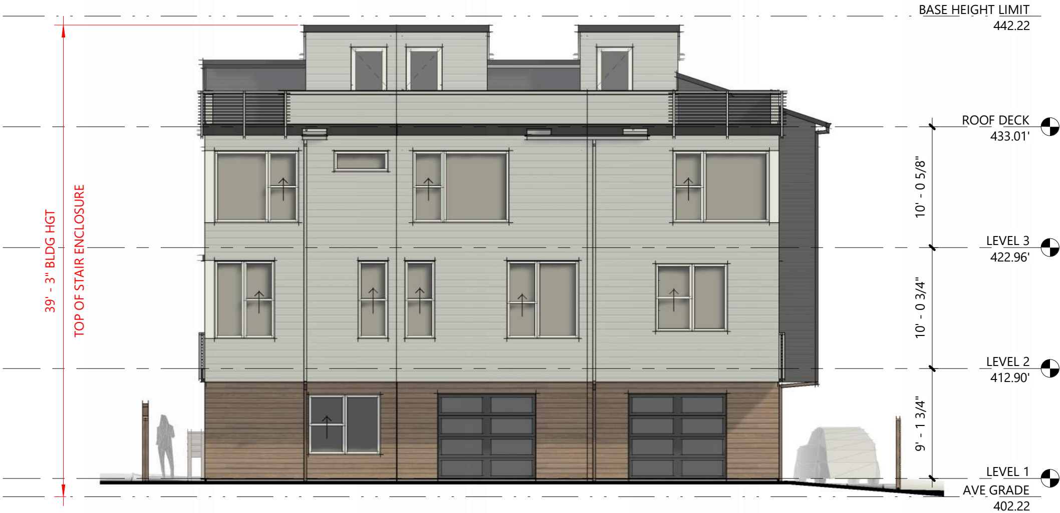
NORTH BUILDING - DRIVE AISLE ELEVATION 1/8" = 1'-0"
