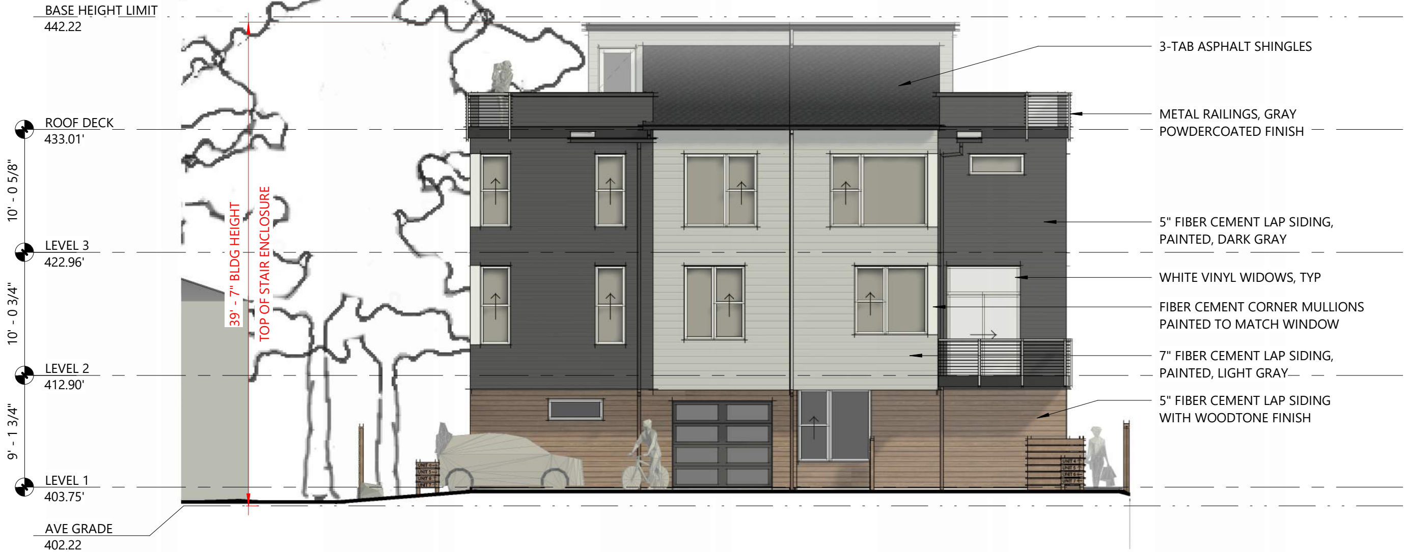
SOUTH BUILDING - DRIVE AISLE ELEVATION 1/8" = 1'-0"
