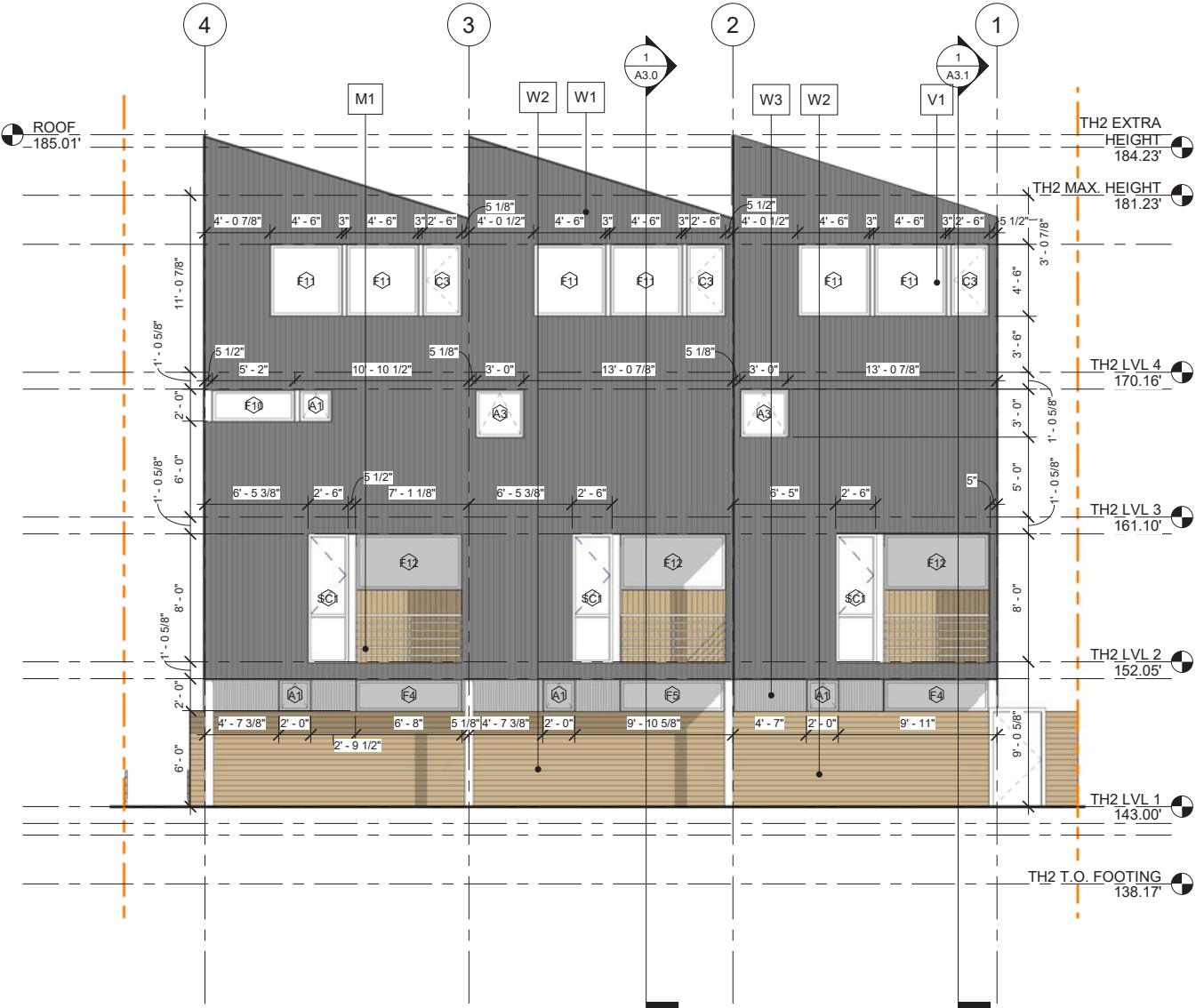
Elevations: East Unit E-Elevation Scale 3/32" : 1' - 0"
