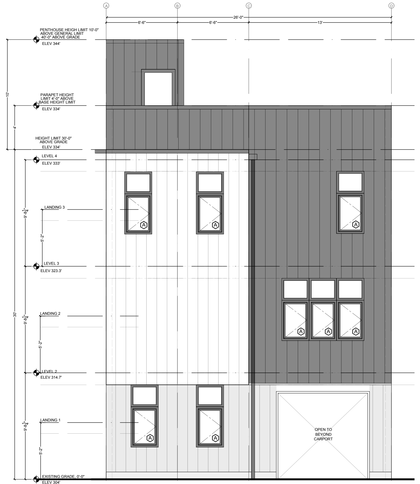
EAST ELEVATION SCALE: 3/16" = 1'-0"
