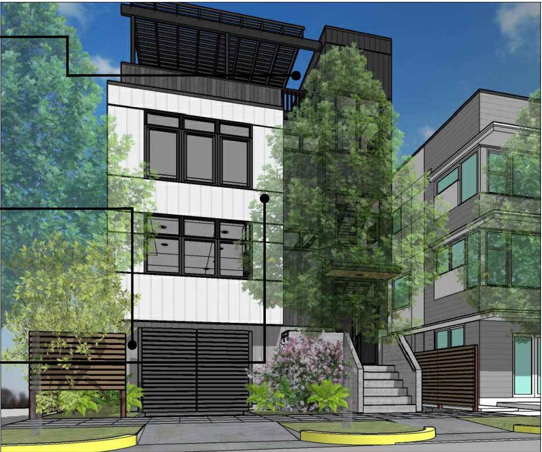
BLACK PAINTED STEEL RAILINGS AND DETAILS, \frac{3}{8} " x 2" FLAT BAR, THROUGHOUT, RAL#9005
