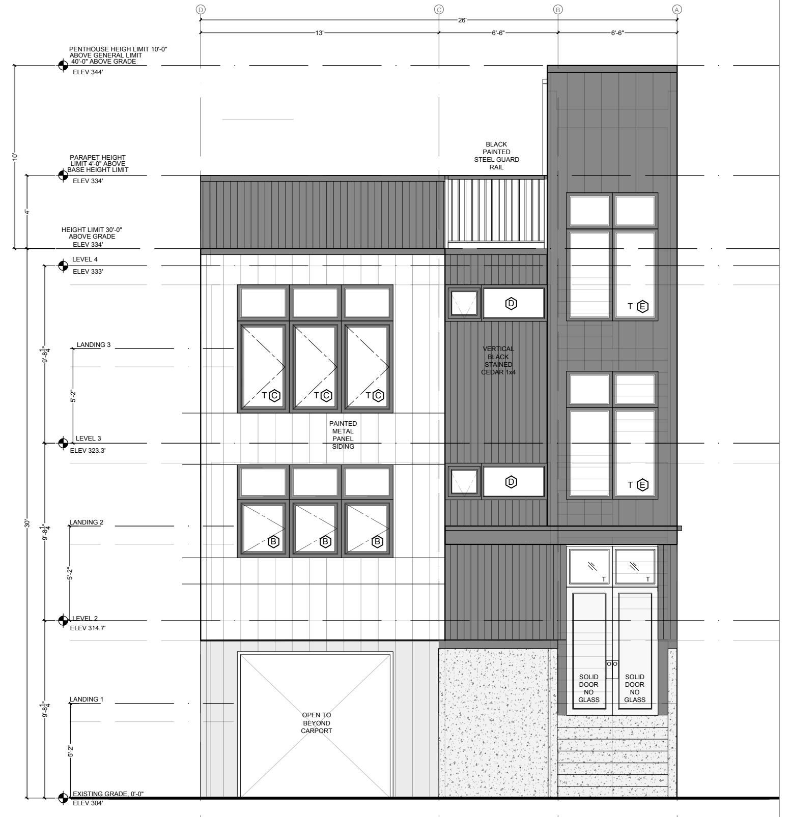
WEST ELEVATION (street facade) SCALE: 3/16" = 1'-0"
