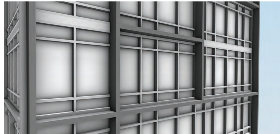
ENLARGEMENT OF WINDOW WALL SHOWING MULLION EXTENSIONS
