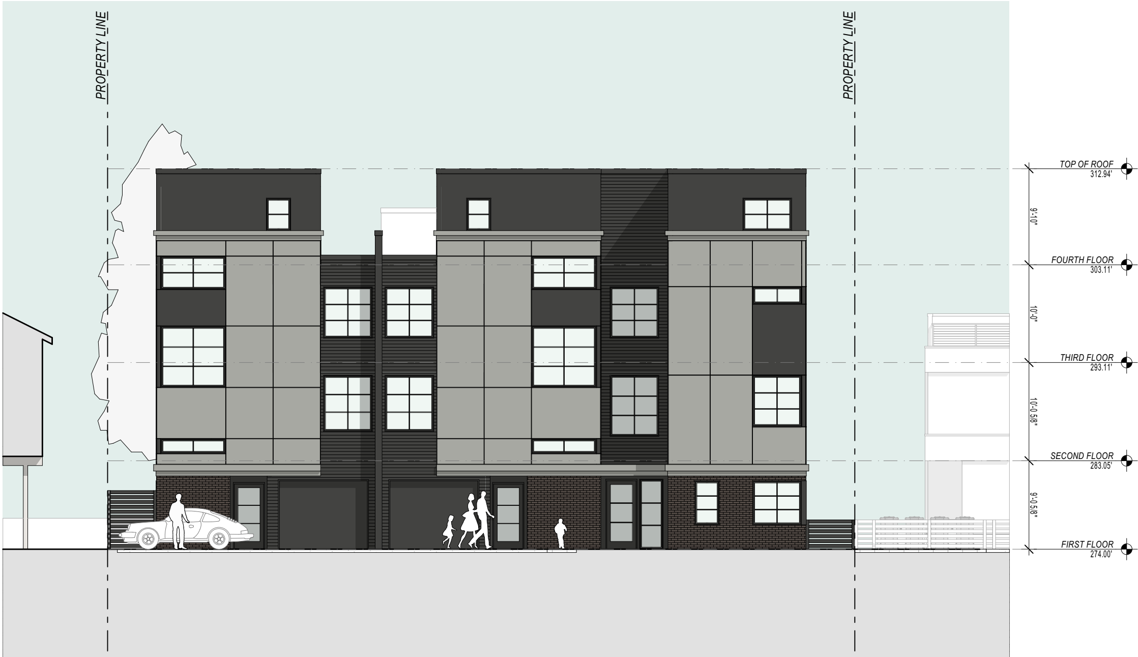
EAST ELEVATION. AT COURTYARD.
