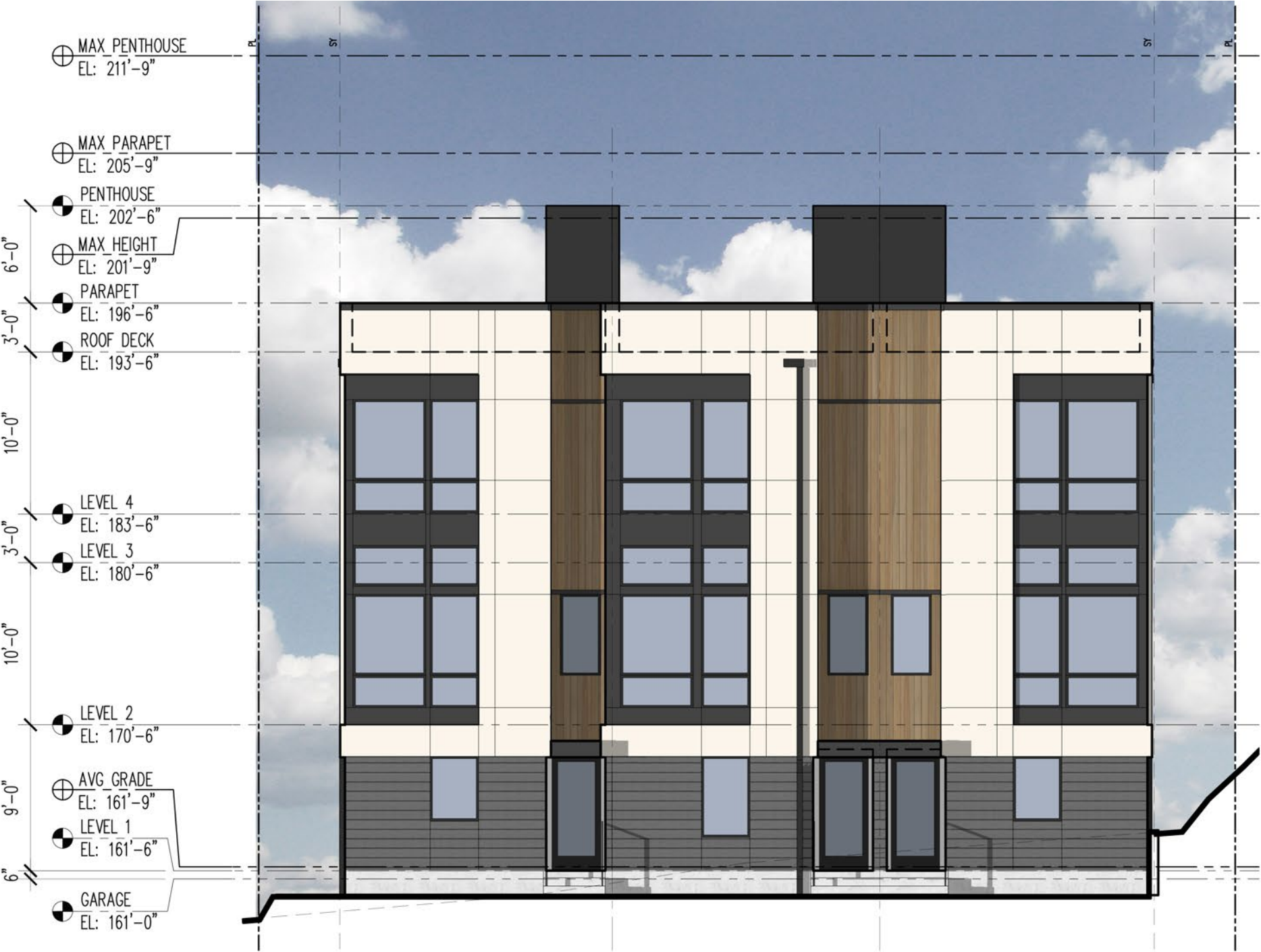
Building 2 - North Elevation SCALE: 1' = 1/8"
