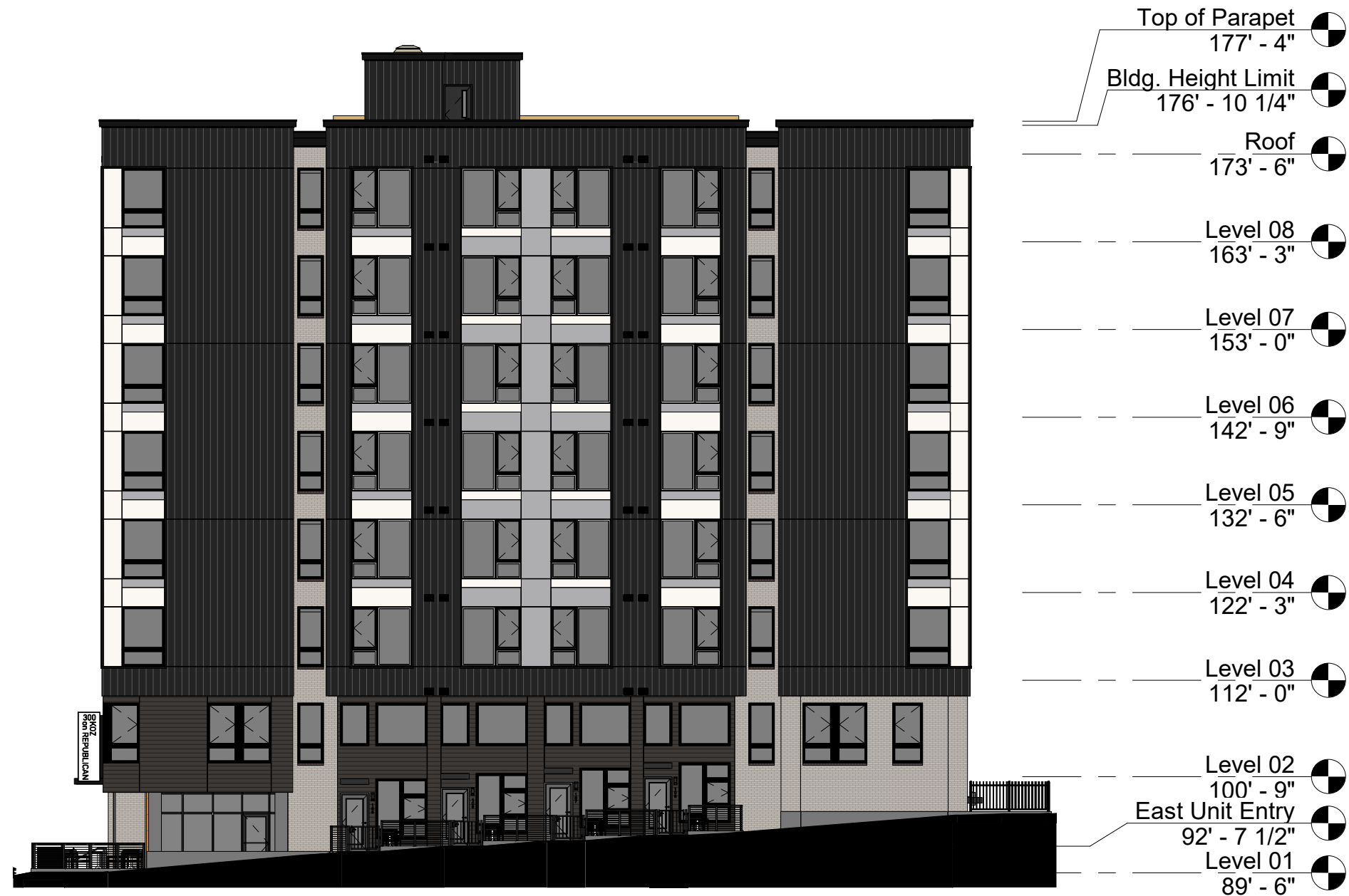
① EAST ELEVATION - Facing 3rd Ave W 1/16" = 1'-0"
