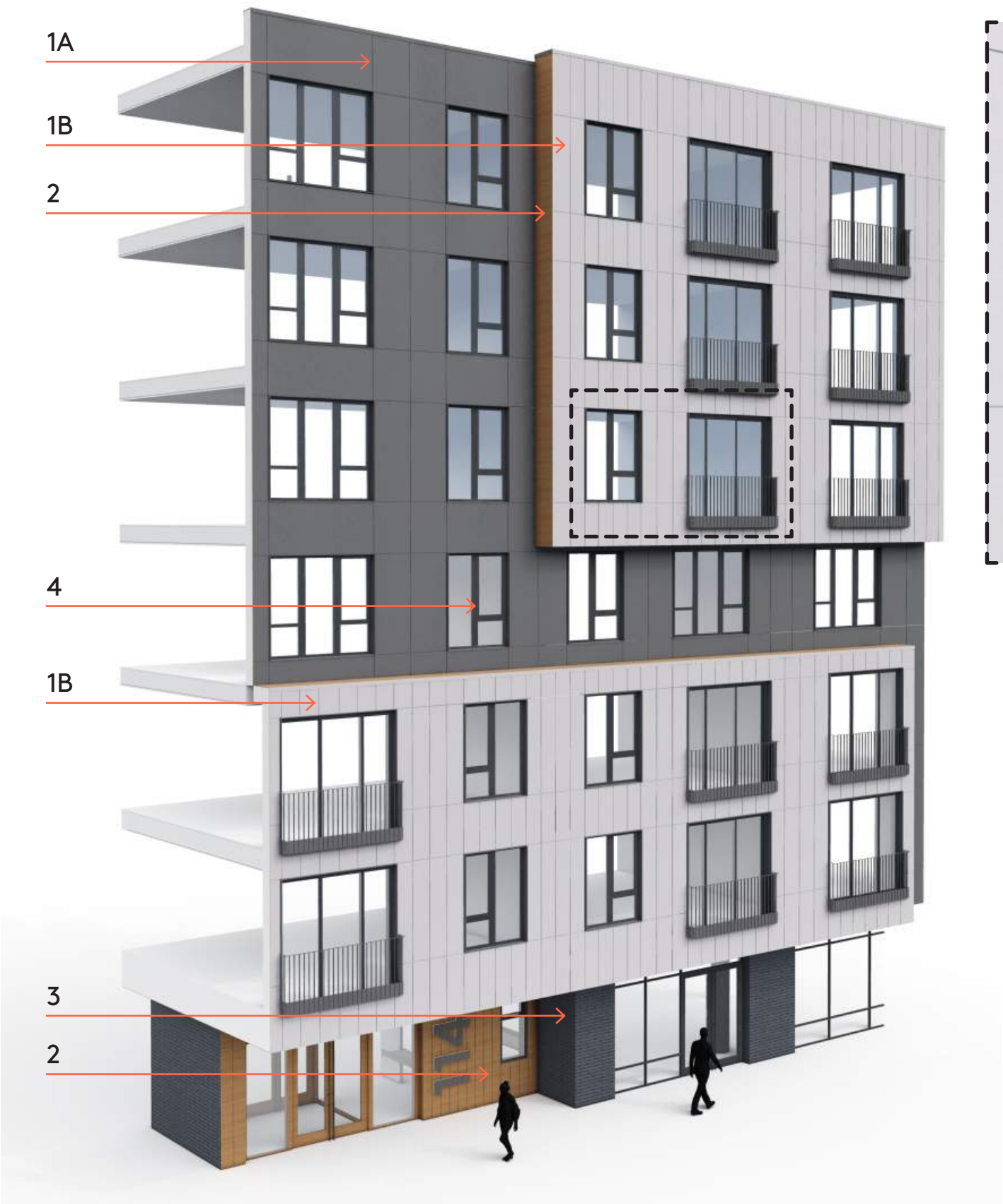
Fiber Cement Panel: Equitone 'Tectiva', TE 85 thru-color
