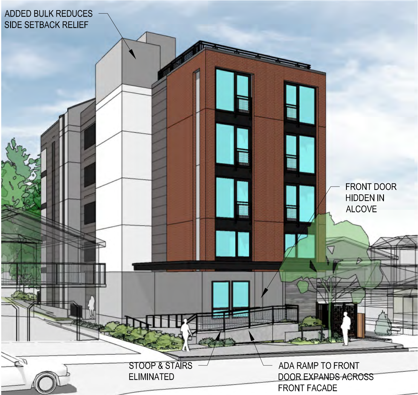
1C EQUIVALENT CODE-COMPLIANT BUILDING N.T.S. N
