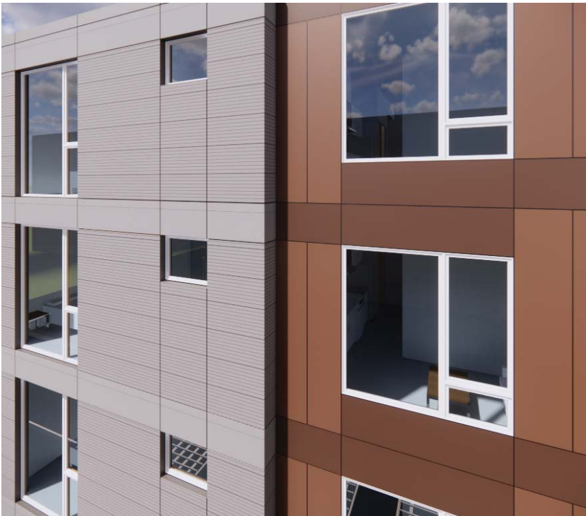
FIBER CEMENT PANEL JOINTING
