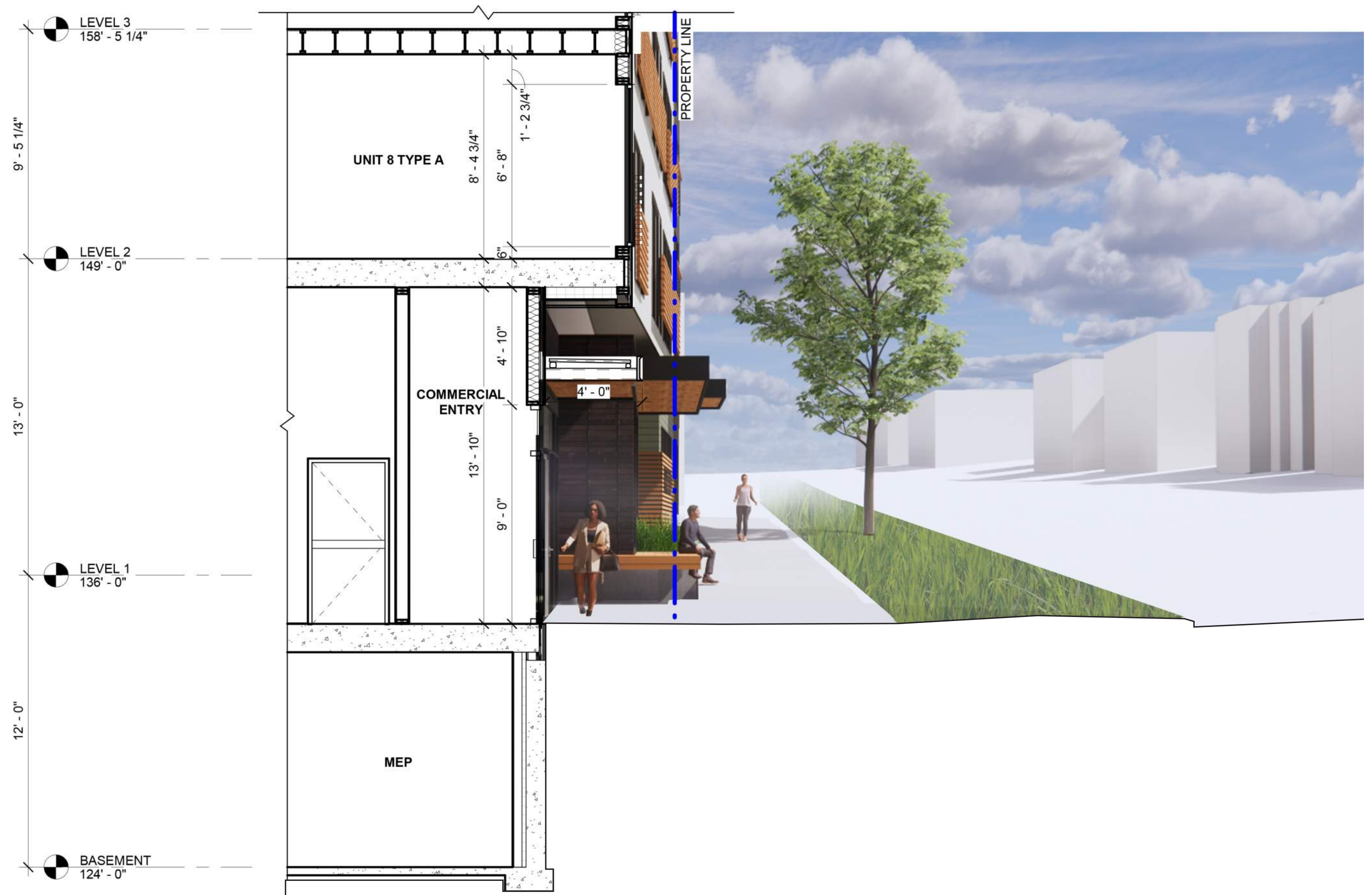
ENLARGED SECTION AT COMMERCIAL ENTRY LOOKING NORTH
