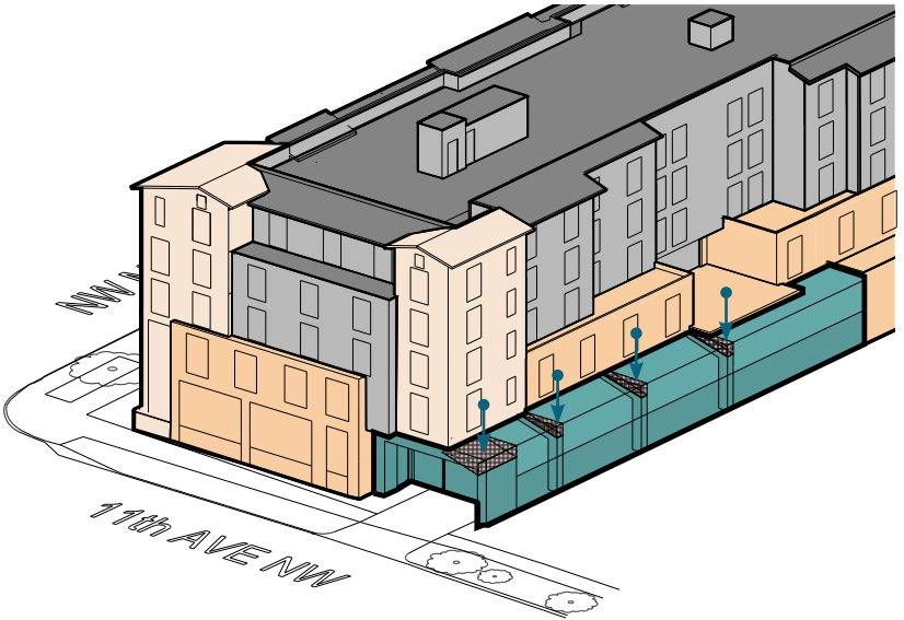
PITCHED - ZONING & SETBACK THE BUTTRESSES ARE PITCHED TO ACCOMDATE HEIGHT AND SET BACK REQUIREMENTS.
