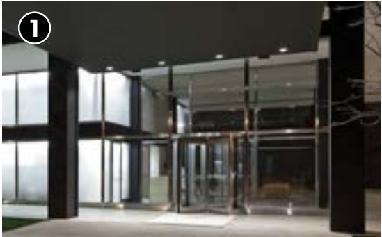
Recessed downlights highlight entries; light source regressed within fixture
