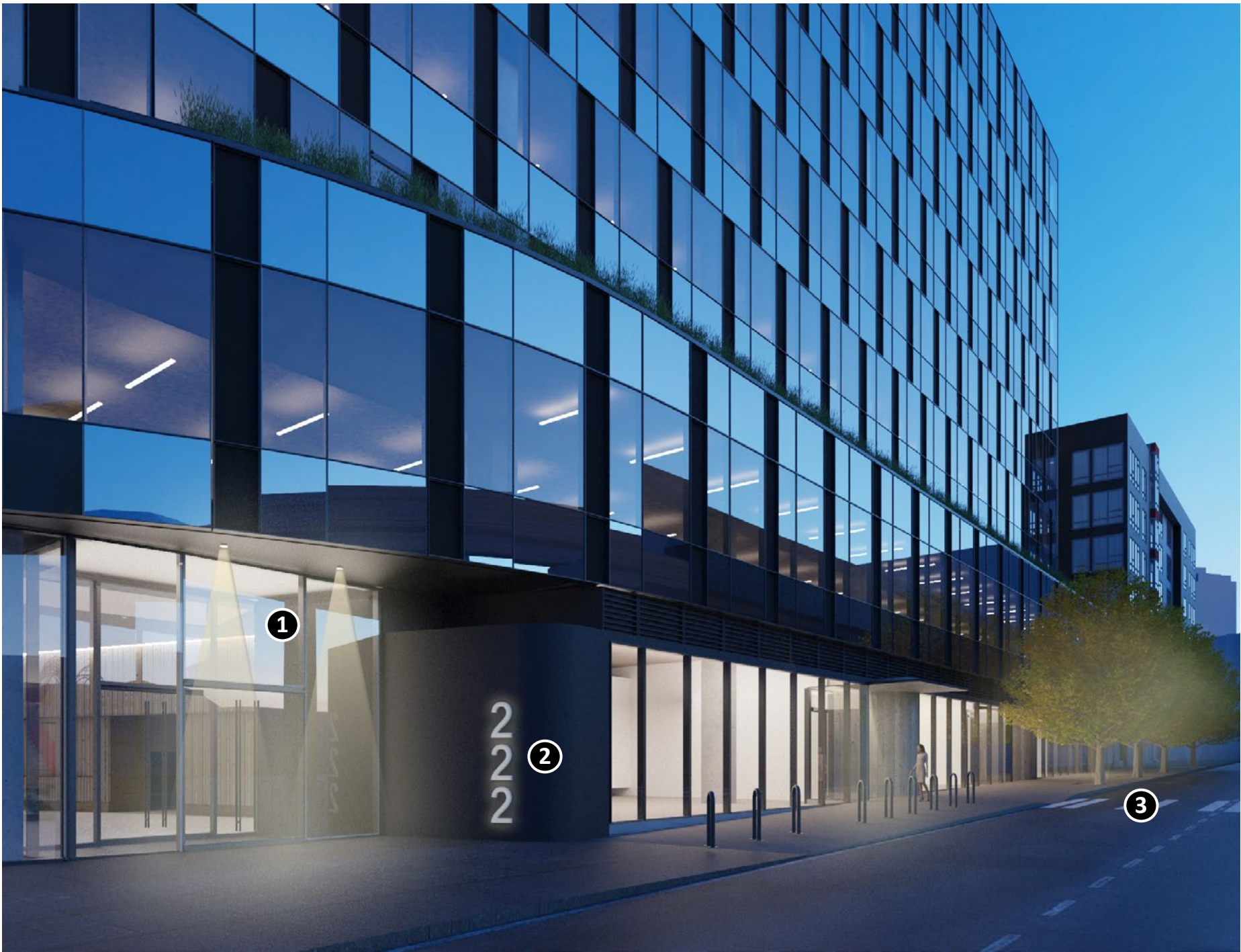
Recessed downlights highlight entries; light source regressed within fixture
