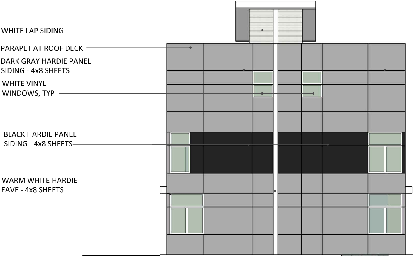
TH UNIT 1&2 SOUTH ELEVATION
