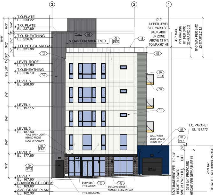
South Building Elevation
