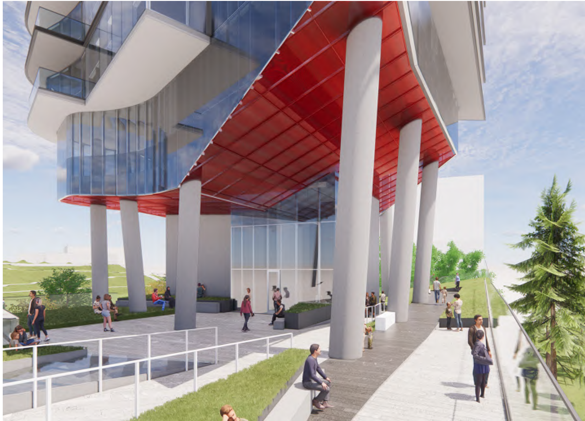
View from Level 2 Plaza Looking at South Tower Soffit - Rendered with Red Tensile Fabric Soffit
