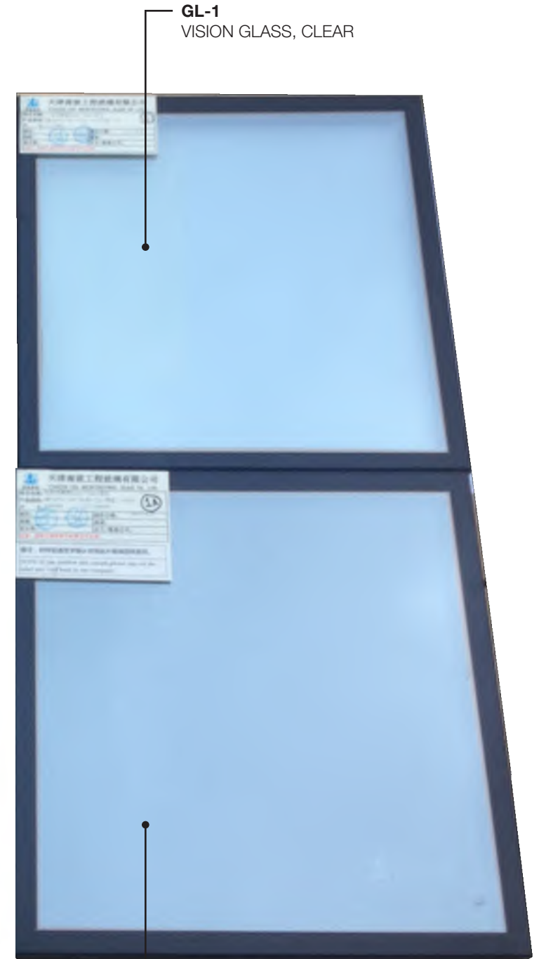
GL-2 SPANDREL GLASS BELOW VISION GLASS FULLY FRITTED #3 SURFACE, DARK COLOR TO MATCH APPEARANCE OF VISION GLASS IN DAYLIGHT
