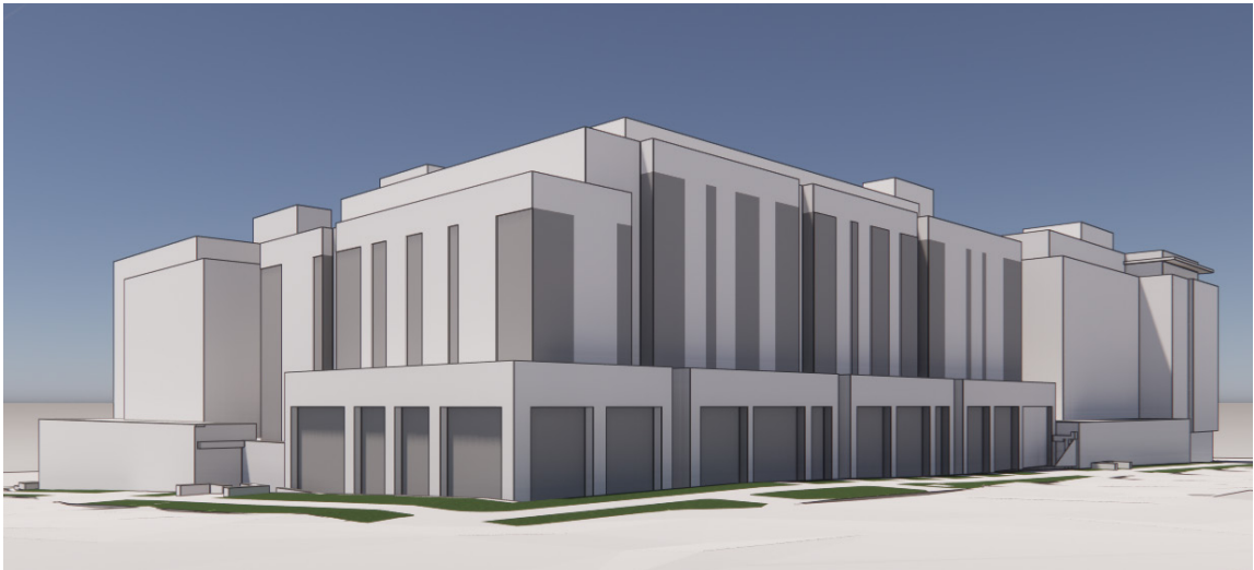
Building B massing refinement: strong ground level massing reinforced with individual openings at the units and upper residential massing forms are reinforced with vertical groupings for windows located at the corners
