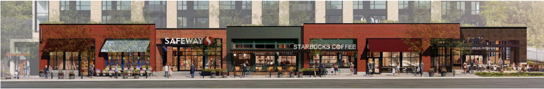
Option 1: 2-1- 1-2-1 Center bay has two varying parapet heights for store entry and the cafe seating. Deli bay parapet is lower than the remainder of the grocer and matches the cafe seating area.
