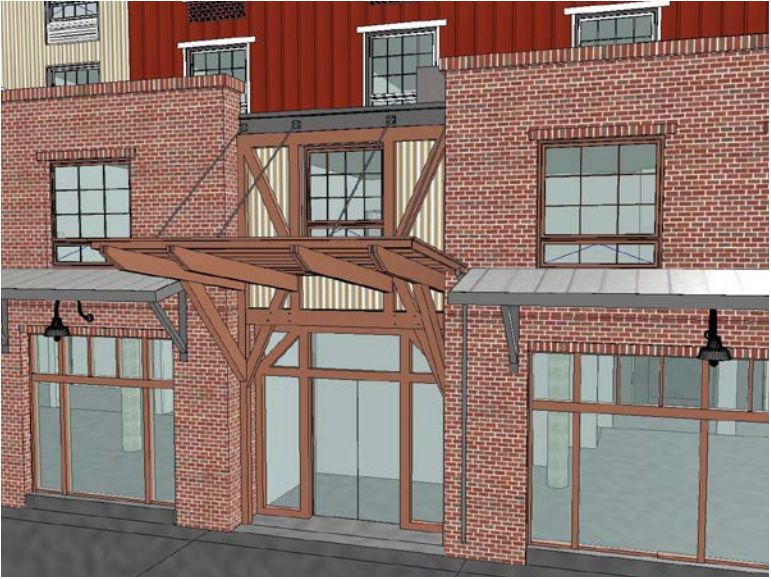
METAL CLADDING WITH TIMBER DESIGN
