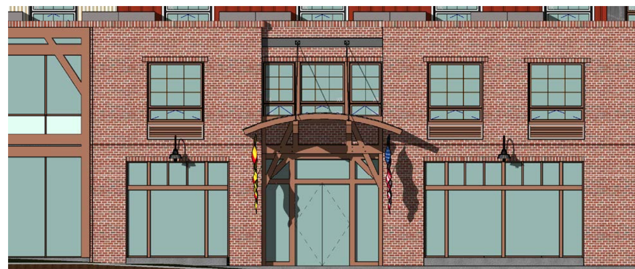
- BRICK CLADDING AT ENTRY
