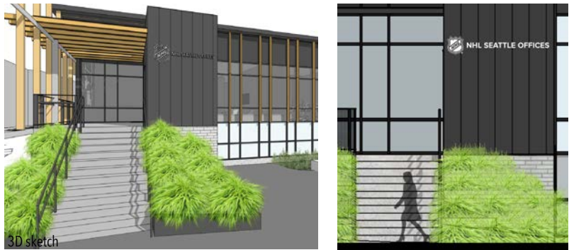
H Wall Sign 2: Installed at 14'-0" above grade Construction: Powder coated aluminum letter bodies and backs with white acrylic face pin mounted to substrate. Size: 2'-2" high by 7'-6" (15.6 SF) Maximum Size Allowed by Code: 672 SF Illumination: 7100 K white LEDs
