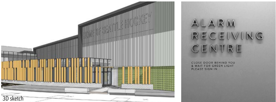
G Wall Sign 1: Installed at 34'-0" AFF Construction: 2.5" deep powder coated aluminum channel letters pin mounted to metal panel wall system; finish to match metal panel system. Size: 4'-8" high by +/- 65'-6" (311 SF) Maximum Size Allowed by Code: 672 SF Illumination: non-illuminated
