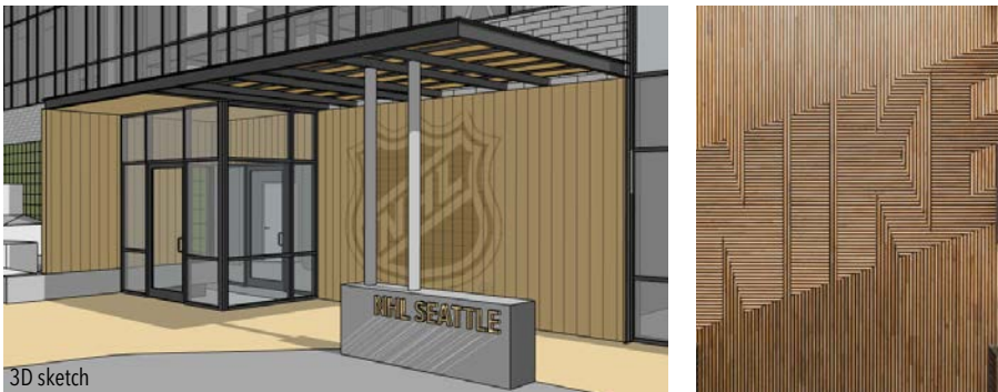
F Branding Sign 2: Channel letters installed at 1'-10" AFF | Logo at 2'-2" AFF to 7'-10" AFF Construction: Halo edge-lit 1/2" deep aluminum channel letters with face finished with wood look. Inset wood logo integral with wood cladding. Size: 9" high text; logo approximately 7'-0" wide Maximum Size Allowed by Code: 672 SF Illumination: 7100 K white LEDs
