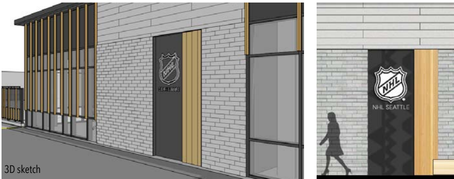
E Branding Sign 1: Installed at 6'-0" to 9'-6" AFF Construction: Powder coated aluminum with gloss-on-matte pattern; wood-look accent; and push through acrylic channel letters / logo. Size: 6'-0" wide sign area Maximum Size Allowed by Code: 672 SF Illumination: 7100 K white LEDs
