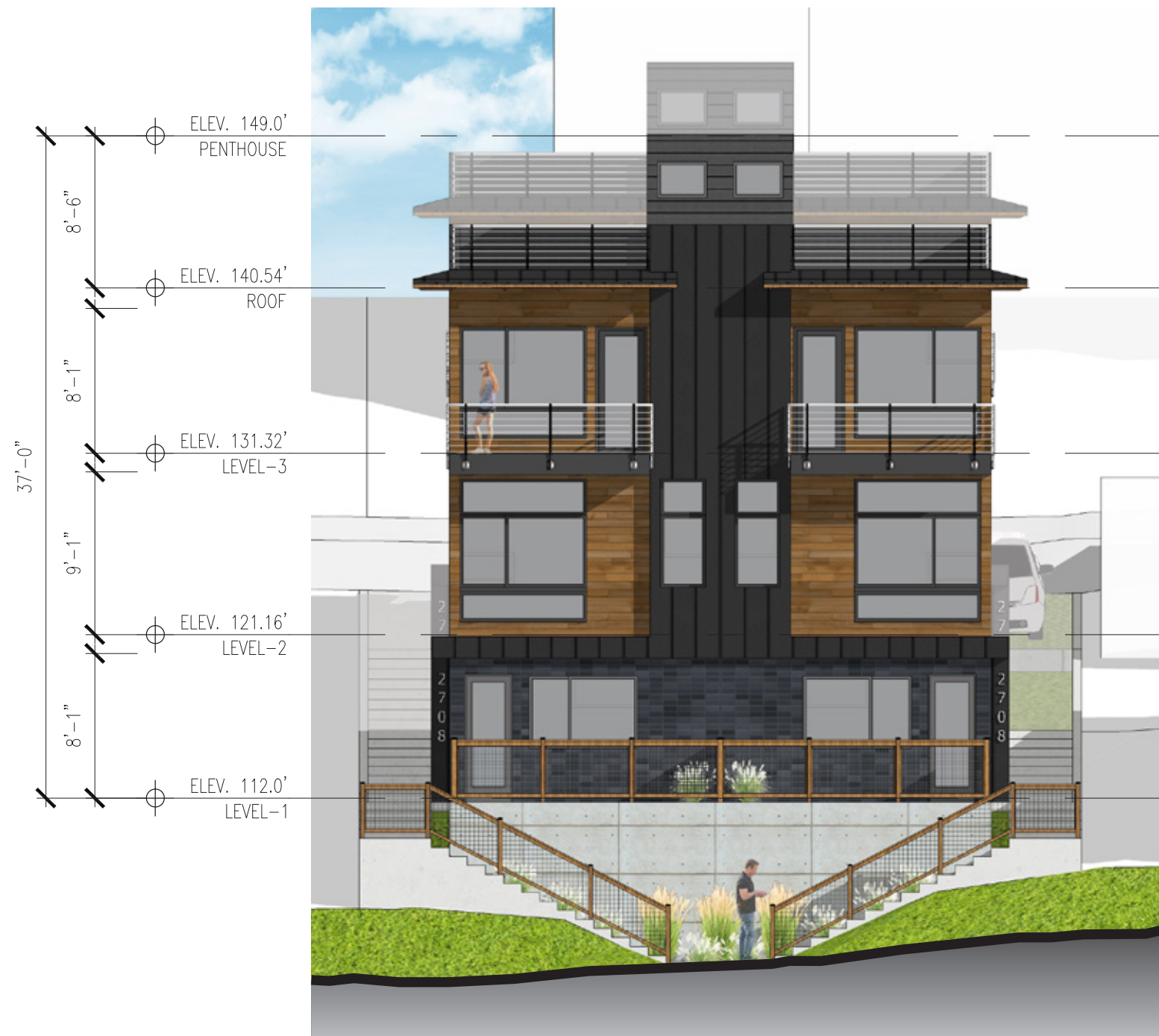
WEST ELEVATION FRANKLIN AVENUE E, FRONT UNITS
