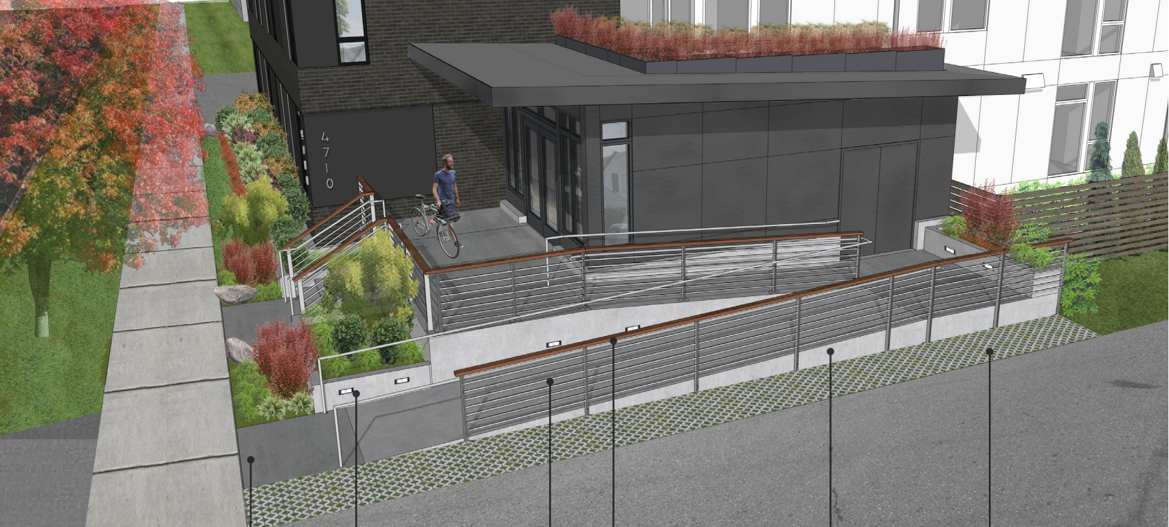
STAINED CONCRETE STEP LIGHT METAL HORIZONTAL RAILING WOOD RAILING CAP CONCRETE PERMEABLE PAVERS
