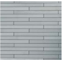
② Cementitious Plank (Rainscreen) Cladding 6" x 72" x 1/2" typical, 5/16" open joints, -polar -two texture finish -integral color
