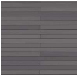
③ Cementitious Plank (Rainscreen) Cladding 6" x 72" x 1/2" typical, 5/16" open joints, -chrome -two texture finish -integral color
