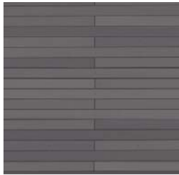
③ Cementitious Plank (Rainscreen) Cladding 6" x 72" x 1/2" typical, 5/16" open joints, -chrome -two texture finish -integral color
