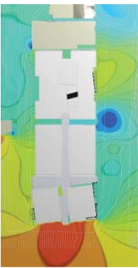
average wind pressure diagram measuring affect of exterior circulation spine to create a protected environment
