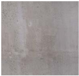
⑥ Cast-In-Place Concrete -light sandblasted architectural finish
