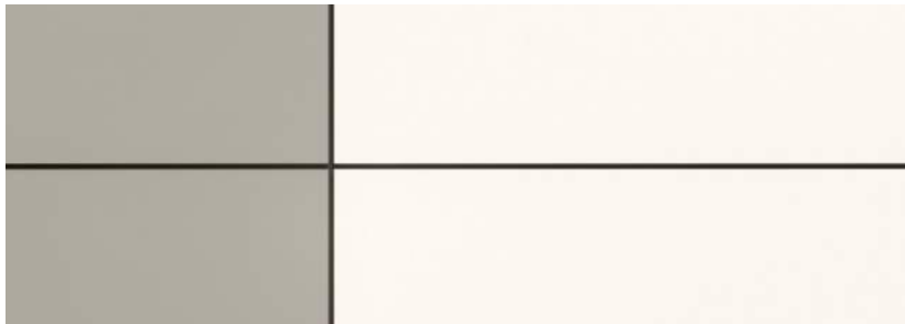
C. FIBER CEMENT ACCENT PANELS • Fiber cement board, painted light gray and cream. • Long panels in running bond configuration. • SW 7016 - Mindful Gray. Acrylic latex exterior paint, satin • SW 7562 - Roman Column. Acrylic latex exterior paint, satin
