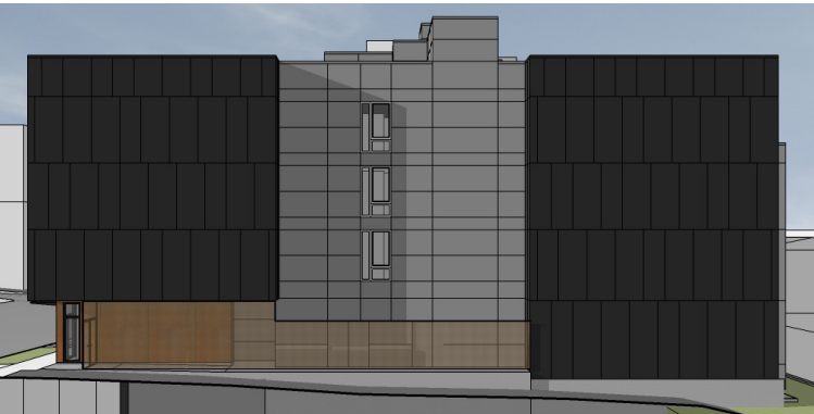
1) EDG SCHEME: CORTEN BASE / DARK ACCENT MASSING / WEST MASSING & MATERIALS VARIED FROM EAST CONCLUSION: NORTH FACADE TOO DARK, NO MATERIAL OR MASSING RELATIONSHIP BETWEEN ELEVATIONS.
