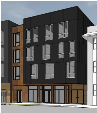
1) EDG SCHEME: CORTEN BASE / DARK ACCENT MASSING / WEST MASSING & MATERIALS VARIED FROM EAST CONCLUSION: NORTH FACADE TOO DARK, NO MATERIAL OR MASSING RELATIONSHIP BETWEEN ELEVATIONS.
