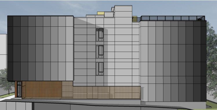
4) CORTEN BASE / DARK ACCENT MASSING / NORTH FACADE GRADIENT STUDY CONCLUSION: TRANSITION NOT SUCCESSFUL, CORTEN WOULD BLEED ON MATERIALS BELOW
