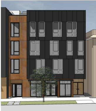
4) CORTEN BASE / DARK ACCENT MASSING / NORTH FACADE GRADIENT STUDY CONCLUSION: TRANSITION NOT SUCCESSFUL, CORTEN WOULD BLEED ON MATERIALS BELOW
