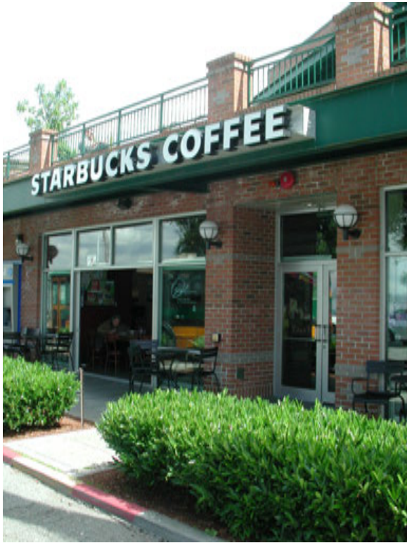
STARBUCKS - 2742 ALKI * BLADE SIGNS, INTERNALLY LIT * RAISED LETTERS ON RACEWAY, INTERNALLY LIT
