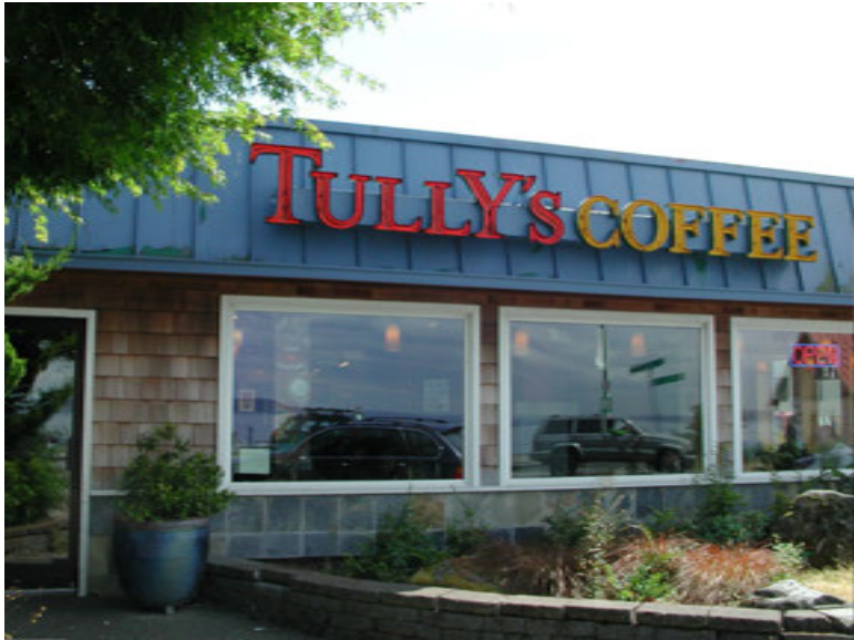
TULLY'S - 2676 ALKI * WALL MOUNTED SIGN, EXTERNALLY LIT * RAISED NEON LETTERS ON RACEWAY
