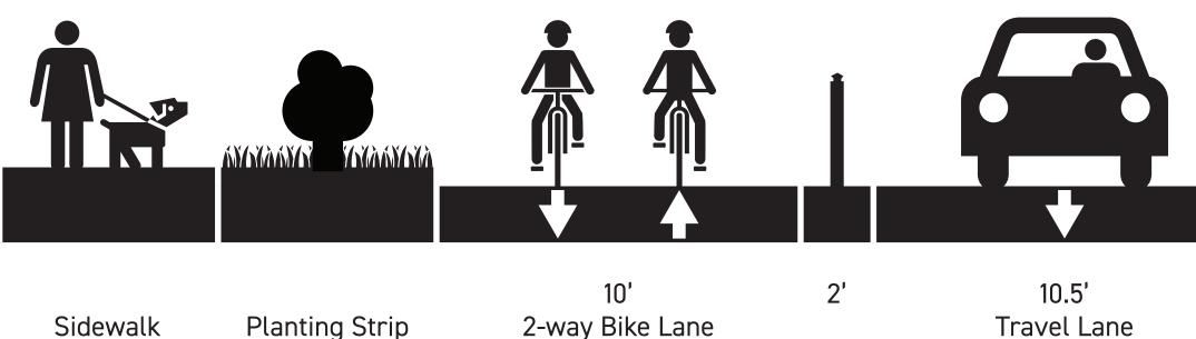
**NOTES:** *Cross sections are looking north.* Street configurations at intersections may look different than cross sections shown. Sidewalk and planting strip widths vary along the corridor.
