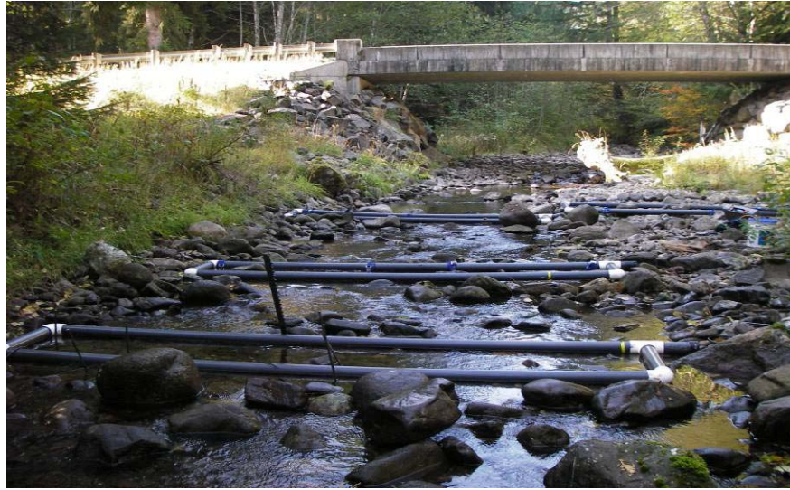
Figure 1.1.—Antenna array at Boulder Creek, October 2005. All antennas were pass-by antennas secured to the streambed by straps held to a combination of rebar stakes, fencing stakes, and anchor bolts in the substrate (antennas 1 and 2 at top of photo).
