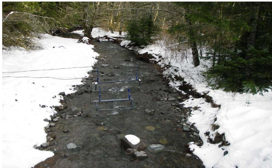
Figure 1.1.—Antenna array at Boulder Creek, October 2005. All antennas were pass-by antennas secured to the streambed by straps held to a combination of rebar stakes, fencing stakes, and anchor bolts in the substrate (antennas 1 and 2 at top of photo).
