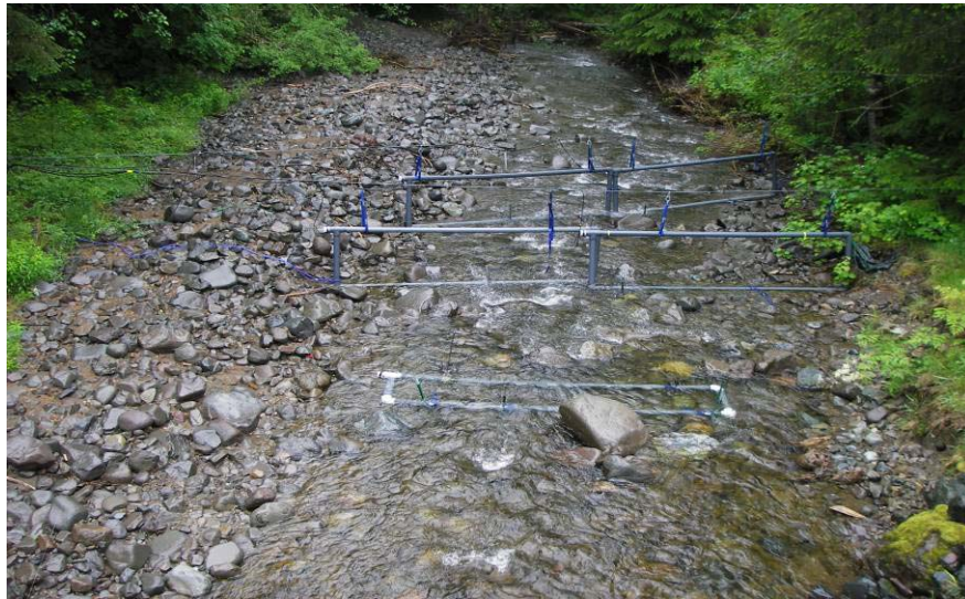
Figure 1.3.—Reinstallation of antennas 1, 3, 4, 5 and 6 at Boulder Creek in June 2006. Antenna 1, configured as a pass-by antenna, was secured to the streambed by straps holding it to fencing stakes driven into the streambed. Antennas 3, 4, 5 and 6 were secured to a cable strung across the streambed in a pass-through configuration.
