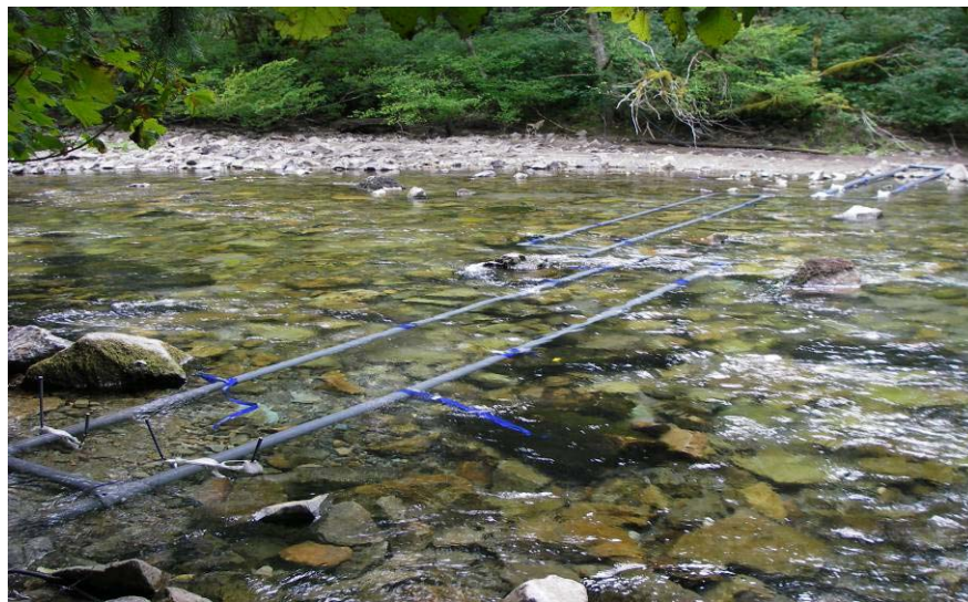
Figure 1.4.—Placement of antennas 1, 2, and 3 (1 at upper right) in the Cedar River, August 2006. Rope and assorted straps secured to a combination of rebar stakes and anchor bolts in larger substrate held the antennas to the streambed.
