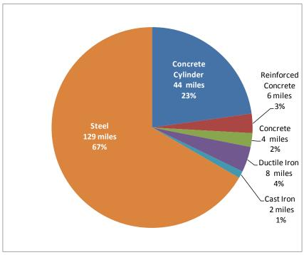
Figure 4-1 Breakdown of Transmission Pipeline Material
