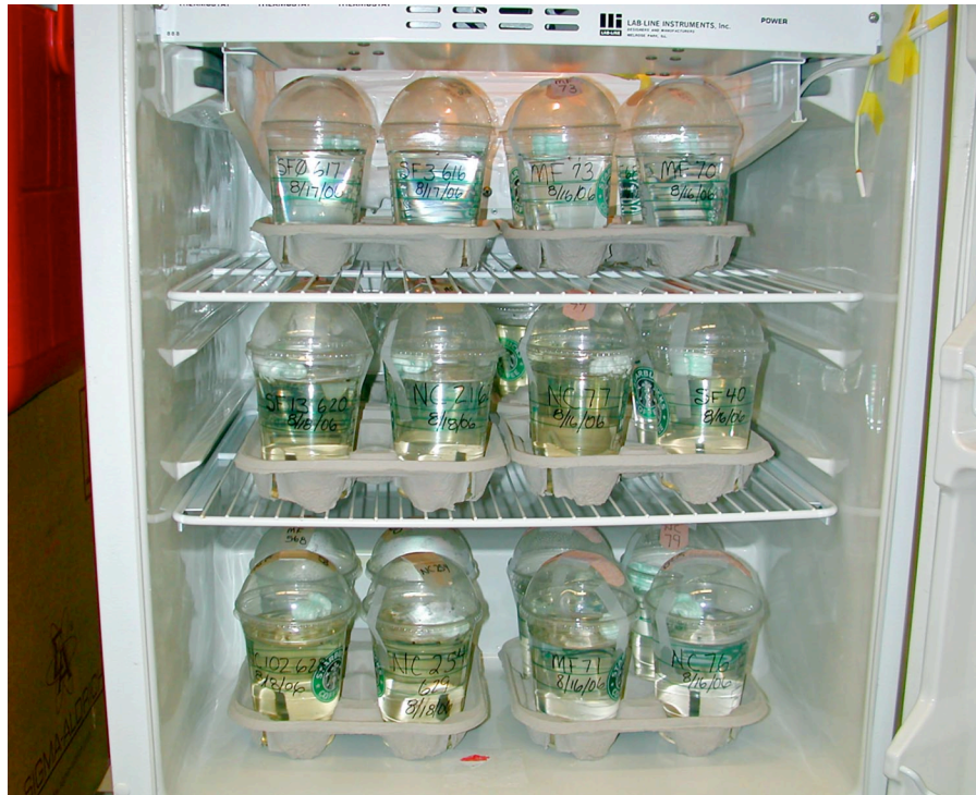
Figure 11. Incubation cups and chamber for assessing the efficacy of Methoprene for controlling the production of mosquitoes in catch basins in Seattle. Larvae were incubated for 5 days at 24-26 C to determine hatching success. Photo: C. Grue
