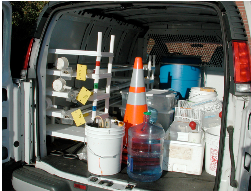
Equipment for monitoring the efficacy and fate of the mosquito larvicides studied in 2006. The 55-gal blue drum constituted a gravity-fed system for rinsing collection gear with de-chlorinated water. Photo: C. Grue
