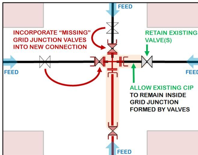
**Single-feed system:** When the new water main segment will form a dead end, or will provide the only standard-diameter supply to an otherwise dead-end area, the grid
