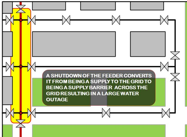
When a larger diameter main interacts with the distribution grid, attention must be given to how potential shutdowns of the large main will affect service to distribution mains, fire hydrants, and water services. Feeder-grid interaction must not defeat the redundancy features incorporated into the distribution grid or increase the shutdown/outage scope experienced by customers served by the grid or served directly off a larger diameter distribution main.
