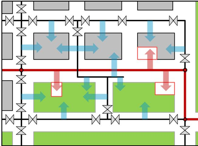
While reducing the number of customers and hydrants supplied by a large-diameter main will reduce the total impact of a shutdown involving the large main, the customers who are affected will experience the lengthier service outage associated with taking a large main out of service. If the shutdown is due to a main failure, repair times associated with a large-diameter main will impose an even greater outage burden on customers directly connected to the large main.
