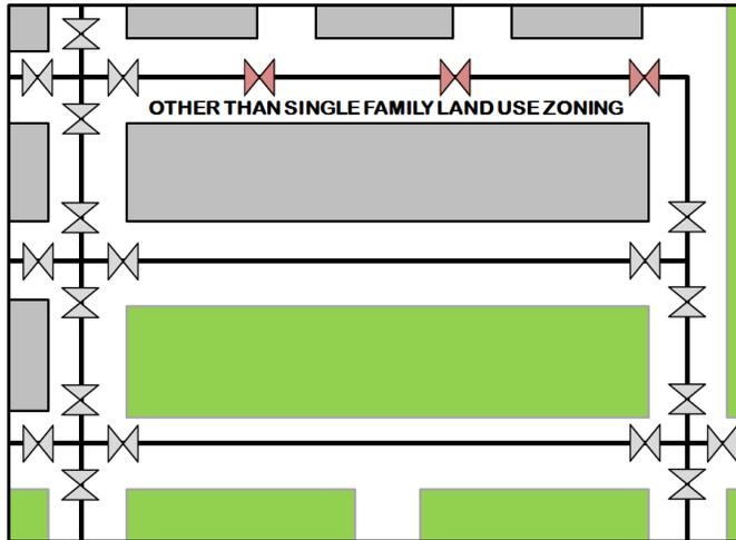
**Single-family residential exception:** In single-family residential (SFR) zones, line valves are required on all water mains approaching a grid junction. However, intermediate line valves between junctions are required only as needed to create water main shutdown segments not to exceed 800 ft in length. See Figure 5-10.
