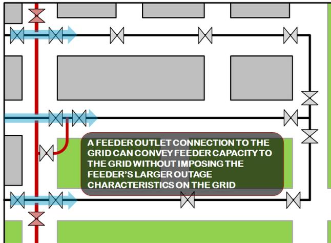
Multiple connections to the grid from different shutdown segments along the feeder can provide the grid with a redundant supply from the feeder that will tolerate a failure and shutdown of the feeder. See Figure 5-16.
