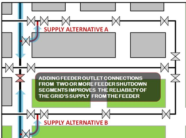
When a large diameter main is fully integrated into the surrounding distribution grid, its higher shutdown/outage implications caused by infrequent valve placement can also be mitigated by avoiding direct customer and hydrant connections to the large main. See Figure 5-17.
