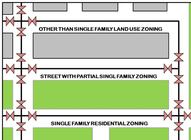
Additional intermediate line valves are required between grid connections, such that any single shutdown segment will be no more than one block or 500 ft in length, whichever is less (except in SFR Zones). See Figure 5-9.
