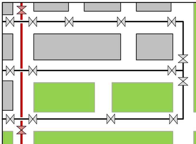
However, if a large diameter main is to be integrated into the water distribution grid, the quarter-mile valve spacing target may be very inappropriate because of its impact on distribution grid shutdown length and outage scope. See Figure 5-13.
