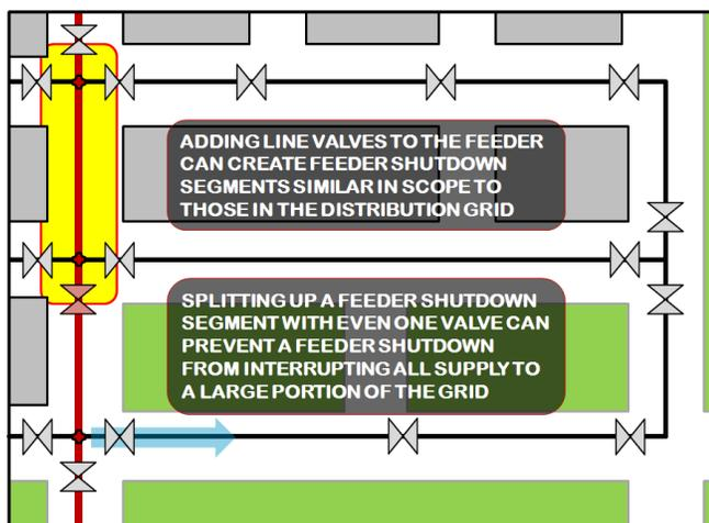
The shutdown/outage implications caused by infrequent placement of costly large-diameter line valves can also be addressed by not fully integrating the large main into the surrounding distribution grid. See Figure 5-15.
