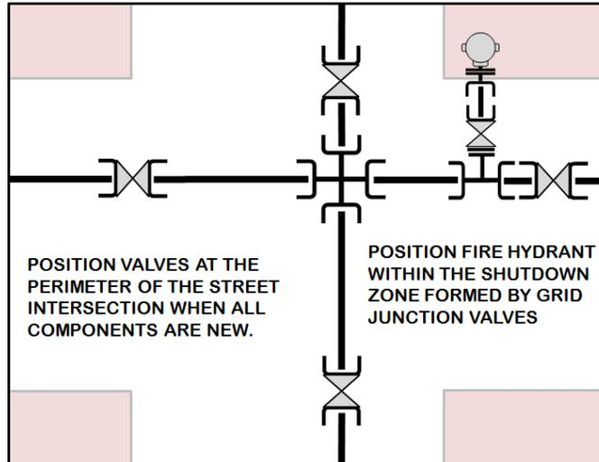
**Looped system:** When the new water main segment will form a supply loop (will receive water from two directions), then any grid junction created by the new water main can utilize the standard intersection valve positioning practices outlined under all-new construction. The new looped main can employ existing valves and existing cast iron pipe located in the intersection of the new junction. See Figure 5-19.
