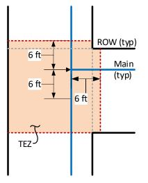
Figure 17-5 TEZ is the Largest Area Created by Valves and Project ROW
