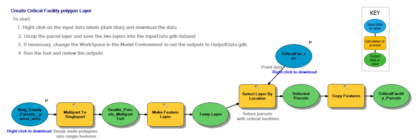
Figure B-3. ArcGIS Model Builder for Developing Critical Facility Area Raster
