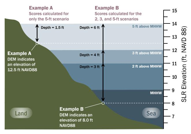
Figure 3-5. Illustration of Depth Estimation for Each Sea Level Inundation Extent
