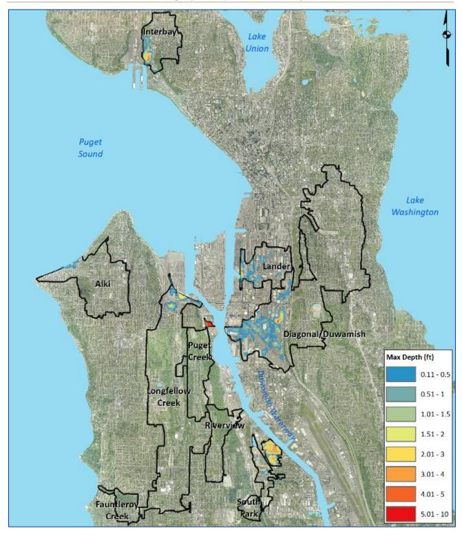
Figure 3-2. Basins and inundation mapping from the CRS
