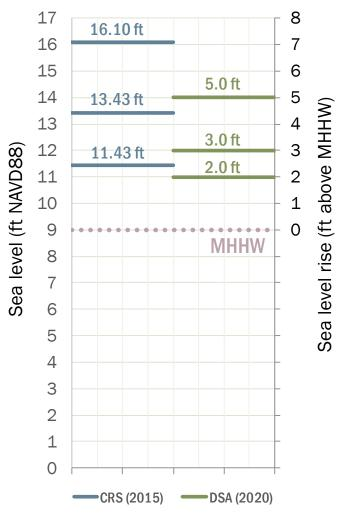
Figure 3-3. SLR scenarios for this study (DSA 2020) compared with sea levels in the CRS SLR added to MHHW of 9.01 ft NAVD88
