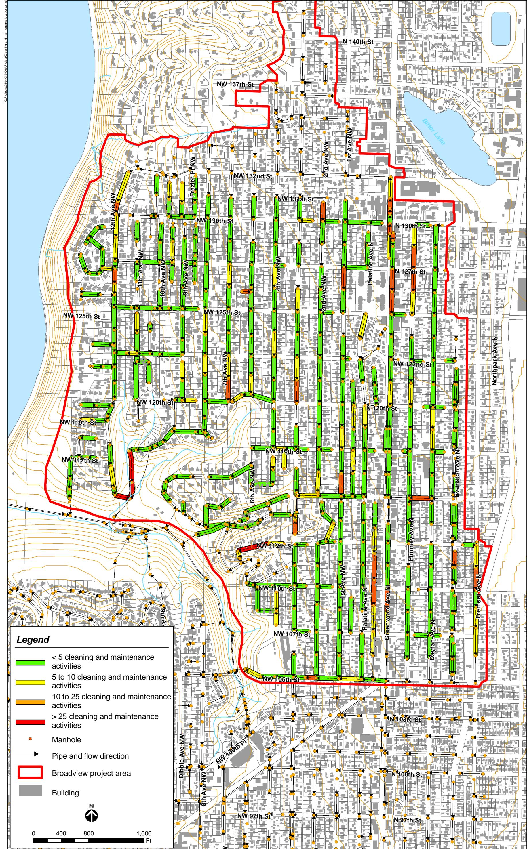
Figure 3. Cleaning and maintenance activity locations and reported occurrences per pipe segment.
