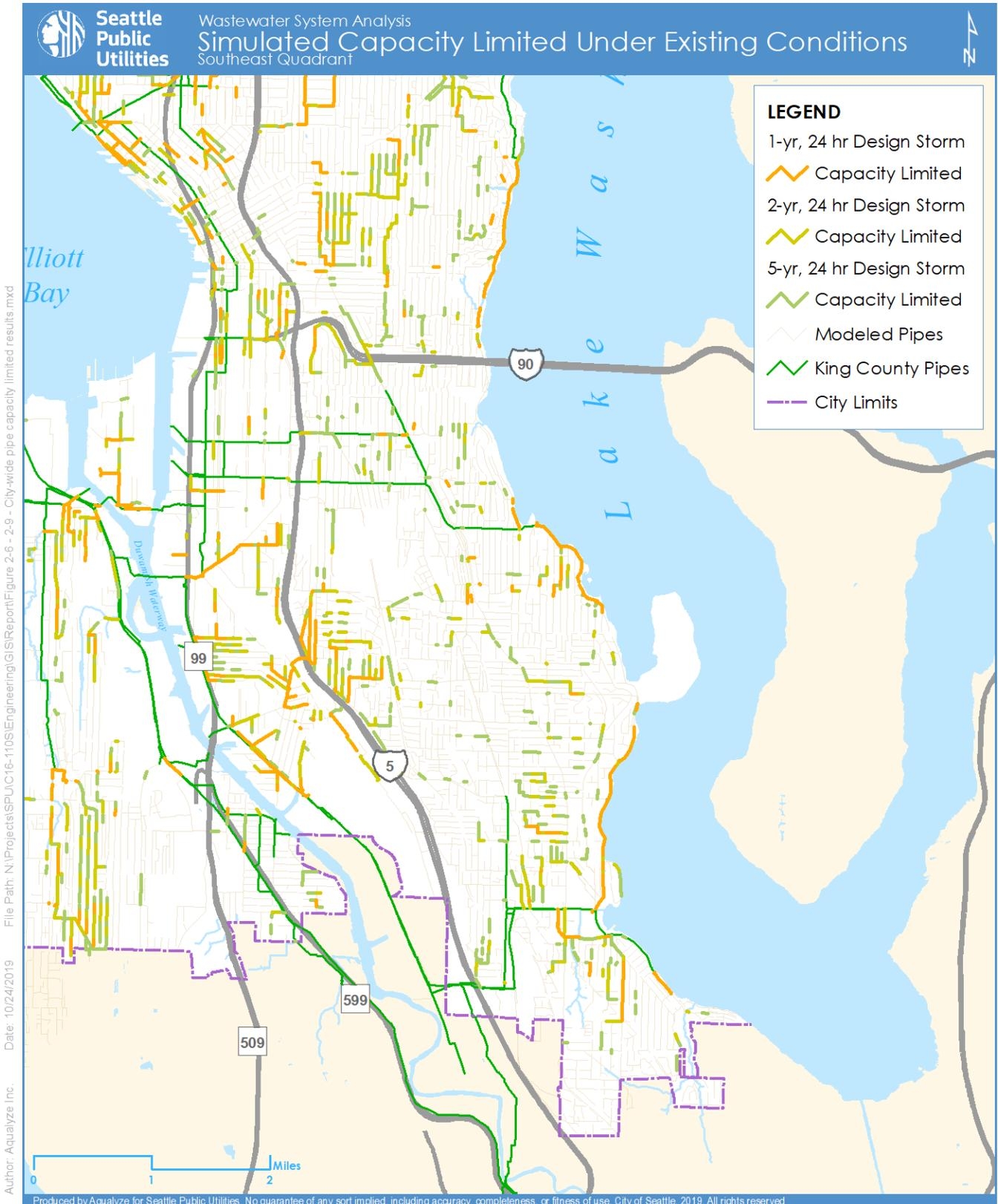
Figure 2-7. Simulated Capacity Limited Under Existing Conditions – Southeast Quadrant
