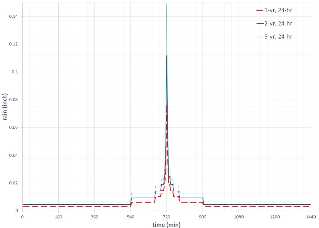
Figure 2-1. Synthetic Design Rainfall Hyetographs
