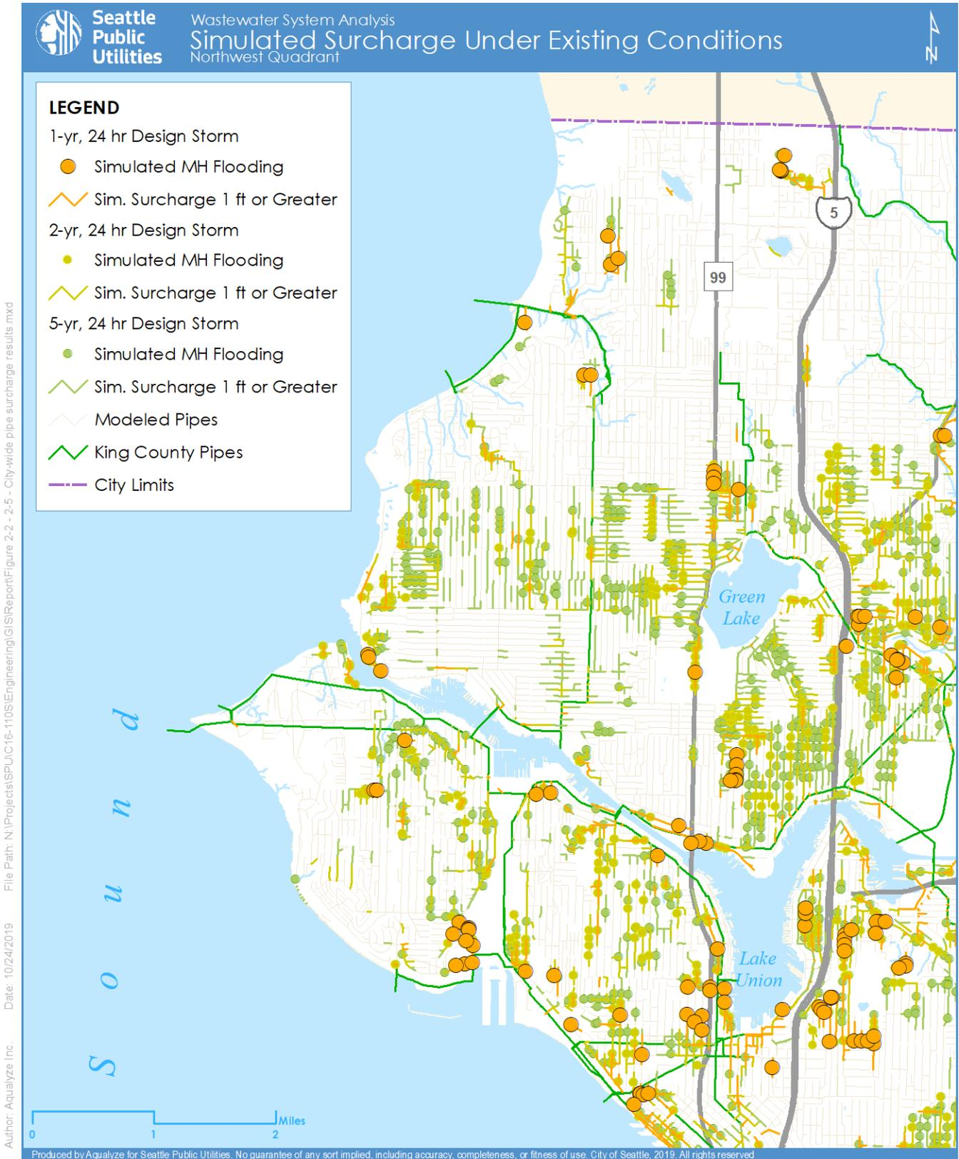
**Figure 2-4. Simulated Surcharge Under Existing Conditions – Northwest Quadrant**
