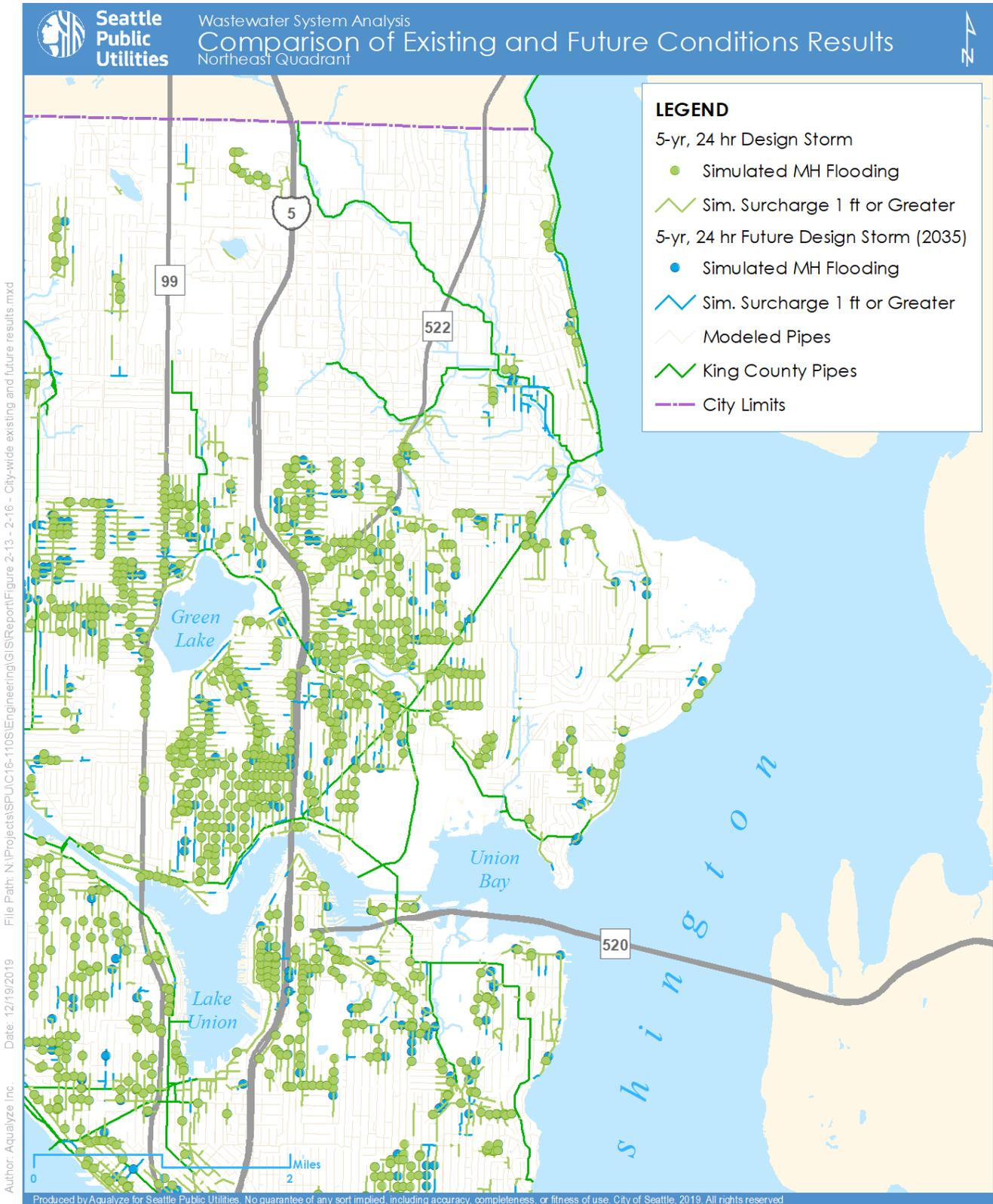
Figure 2-16. Comparison of Existing and Future Conditions Results – Northeast Quadrant
