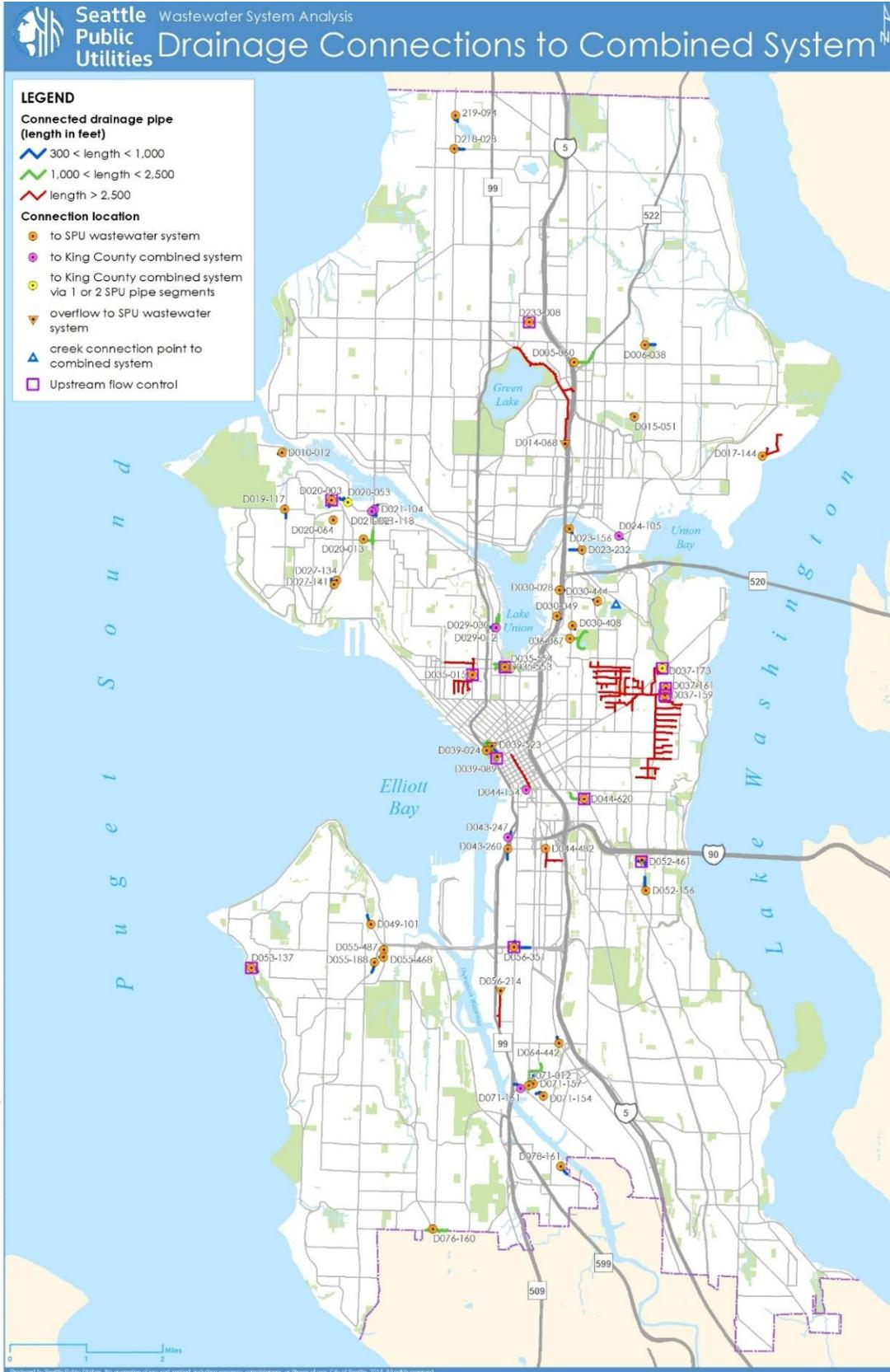
Figure 5-1. Drainage Connections to the Combined System
