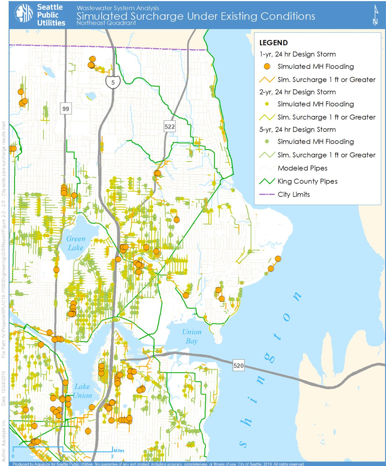
Figure 2-5. Simulated Surcharge Under Existing Conditions – Northeast Quadrant
