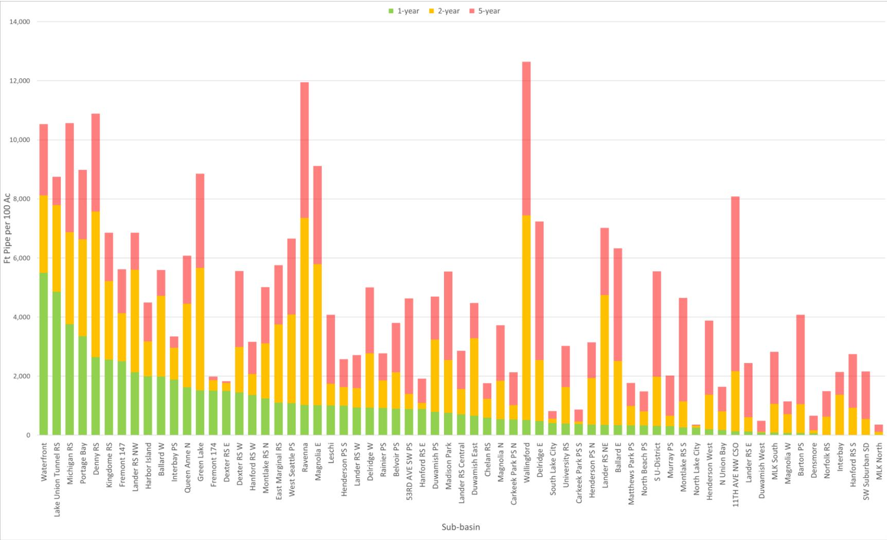
Figure 2-11. Surcharged Pipe Length by Sub-basin Normalized by Area
